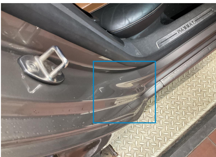
16. Pillar / Back Right Bodywork / Dent / Dent -
