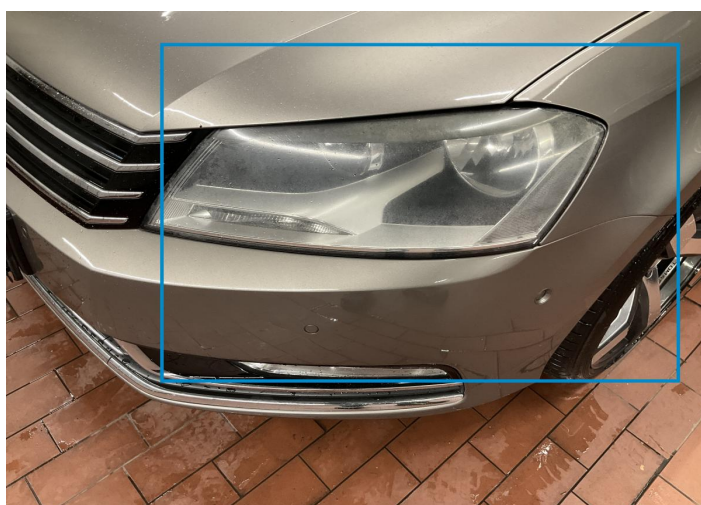
5. Front Light / Front Left Glass Break -
