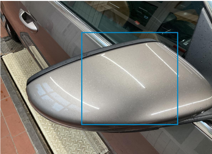
19. Mirror Shell / Front Right Paint / Scratch / Scuff -
