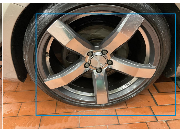
6. Rim / Front Left Out of Bodywork / Scratch -
