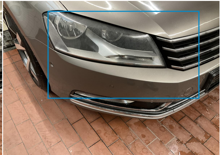
22. Front Light / Front Right Glass Break -
