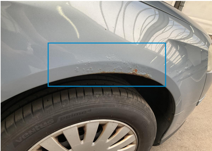
4. Fender / Front Right Paint / Corrosion -
