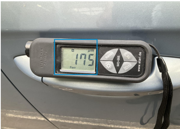
1. Door / Front Right Paint / Poor Previous Repair -
