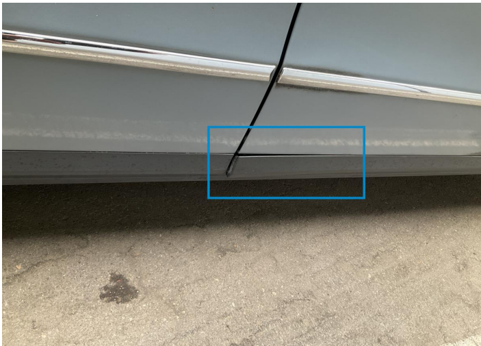
5. Door Side Molding / Front Right Bodywork / Dent / Deformation -
