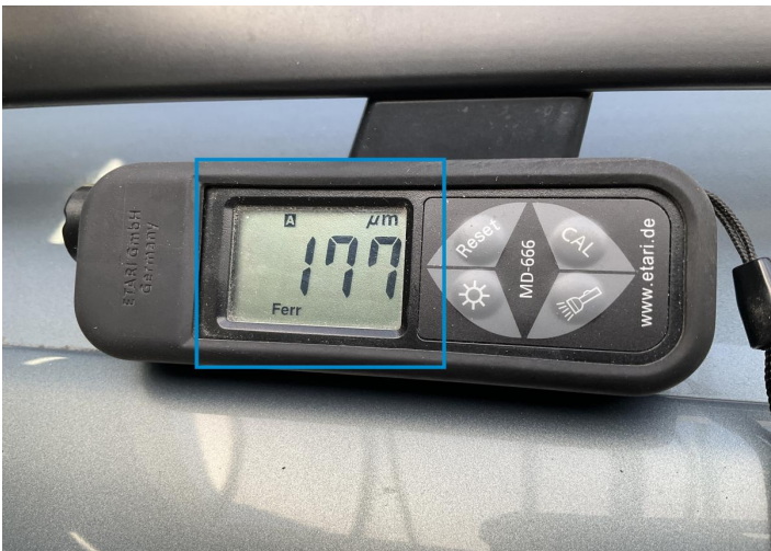
2. Side Panel / Back Right Paint / Poor Previous Repair -
