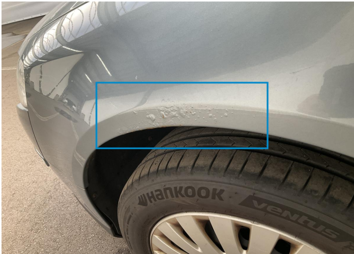
3. Fender / Front Left Paint / Corrosion -
