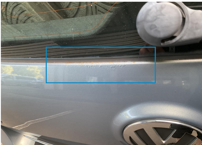
12. Tailgate Paint / Corrosion -
