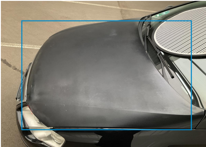
3. Hood Paint / Poor Previous Repair -
