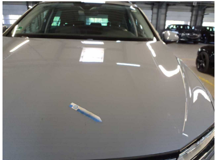
Damage 3: Bonnet: Bonnet - Stone chips - Paint
