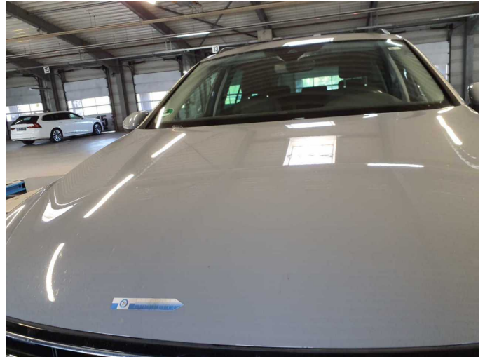
Damage 3: Bonnet: Bonnet - Stone chips - Paint
