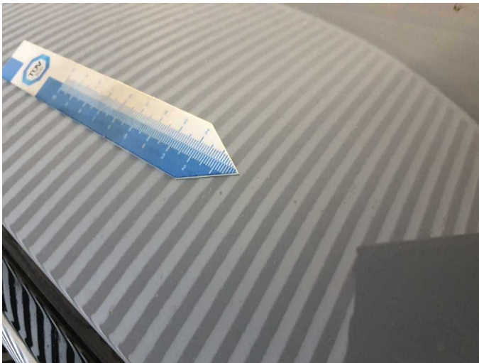
Damage 3: Bonnet: Bonnet - Stone chips - Paint
