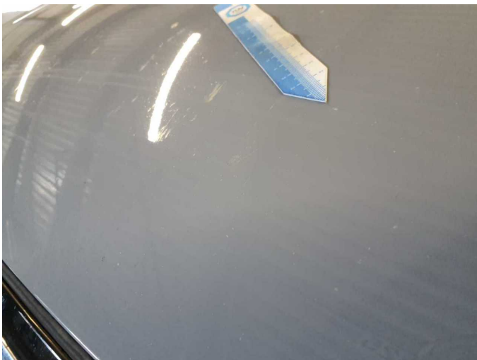
Damage 3: Bonnet: Bonnet - Stone chips - Paint
