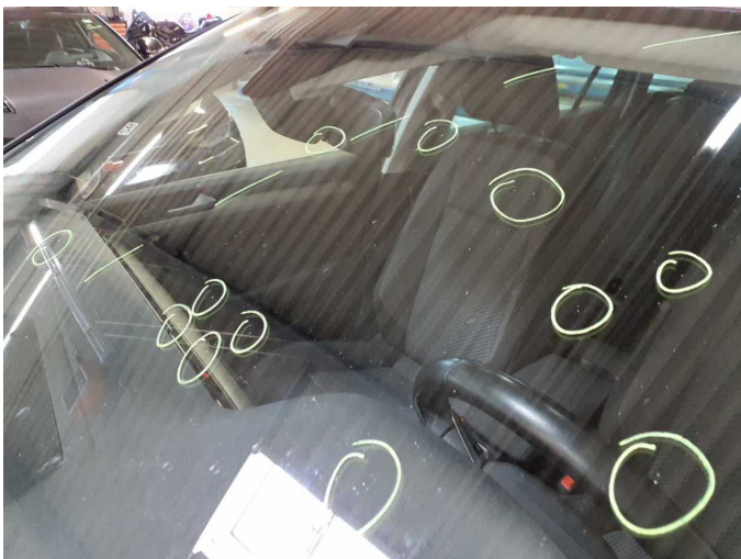
Damage 7: Vehicle glazing: Windscreen (Sandstrahleffekt) - Stone chips - repair according to calculation
