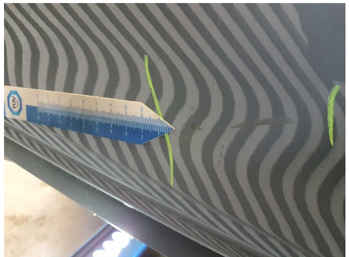
Damage 4: Rear bumper: Rear bumper (+Delle) - Scratched - Repair and paint
