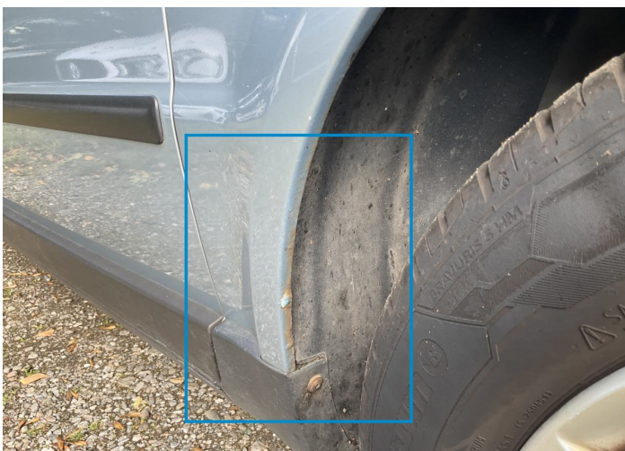
2. Fender / Front Right Paint / Corrosion -
