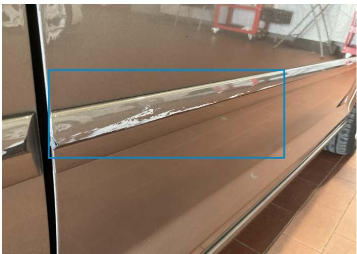
13. Door Side Molding / Front Right Paint / Scratch / Scuff -
