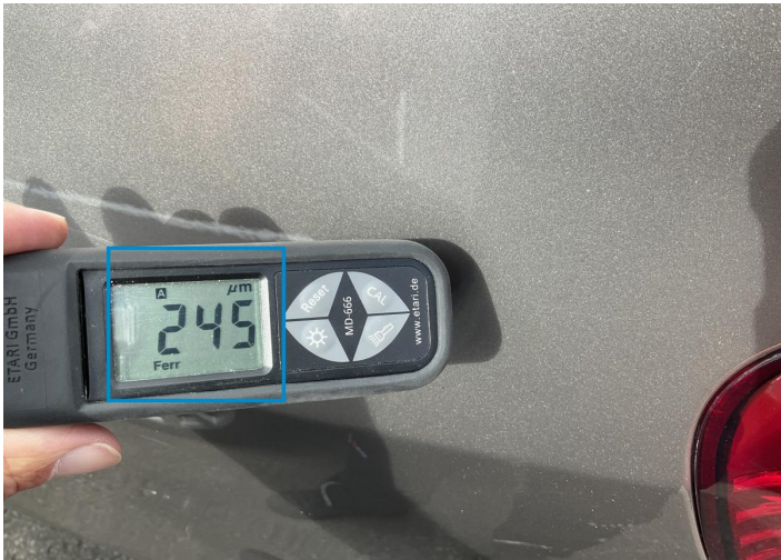
33. Side Panel / Back Left Paint / Poor Previous Repair -
