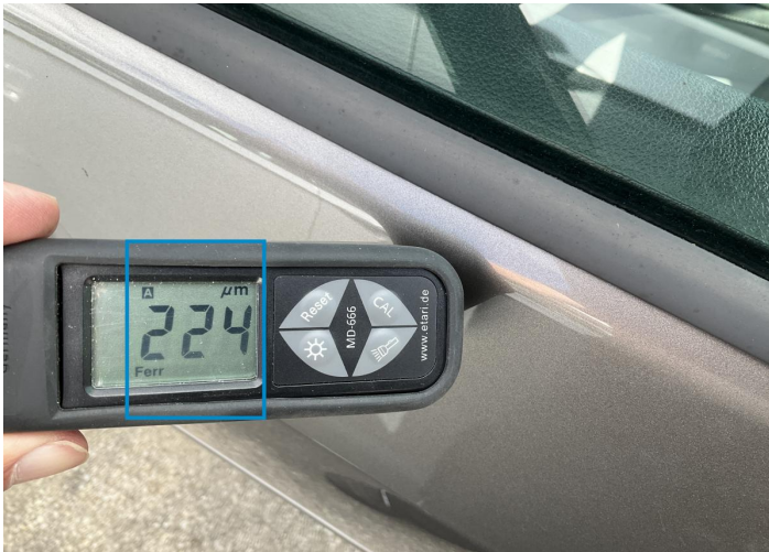
37. Door / Front Right Paint / Poor Previous Repair -
