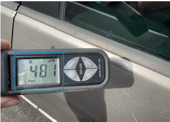
32. Door / Back Left Paint / Poor Previous Repair -
