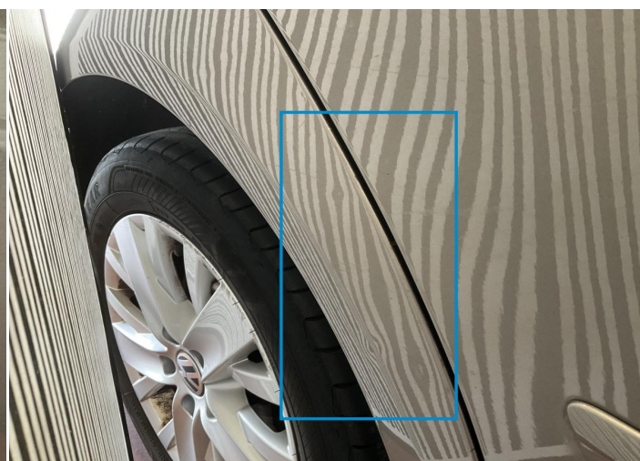
28. Side Panel / Back Right Bodywork / Dent / Dent -
