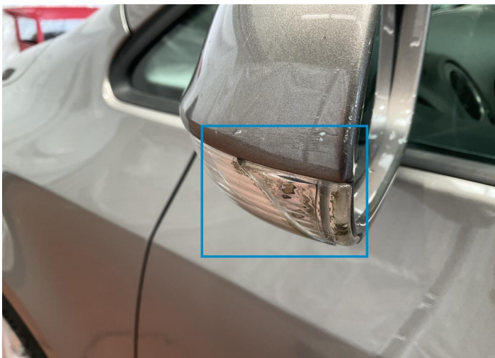
18. Mirror Repeater / Left Glass Break -
