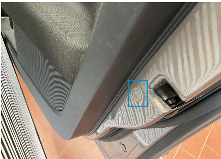
9. Door / Front Right Bodywork / Dent / Dent -
