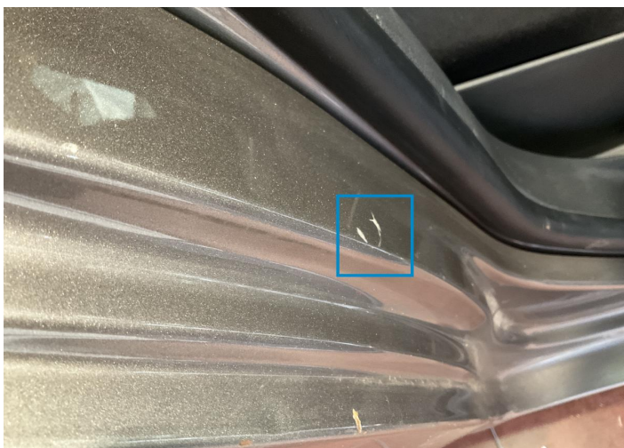
11. Pillar / Back Right Paint / Scratch / Scuff -
