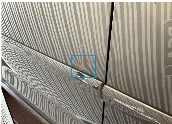
25. Door / Back Right Bodywork / Dent / Dent -
