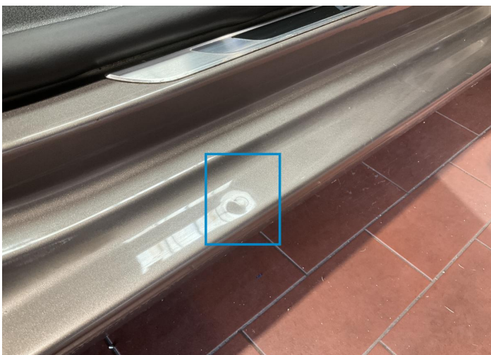
8. Rocker Panel / Center Right Bodywork / Dent / Dent -
