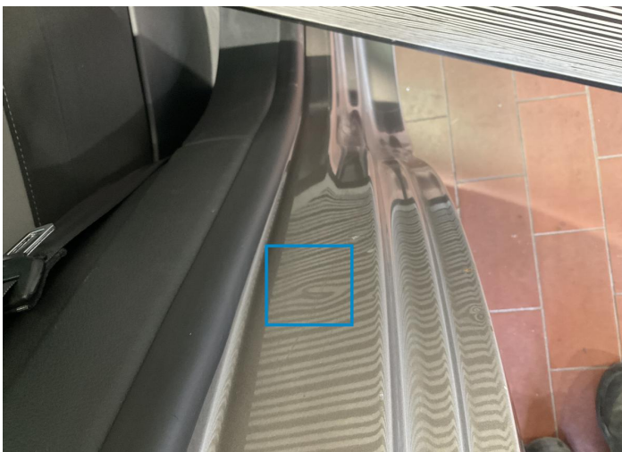
10. Door / Back Right Bodywork / Dent / Dent -
