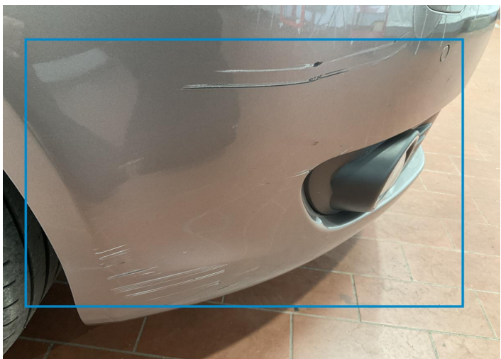
15. Bumper / Front Paint / Scratch / Scuff -
