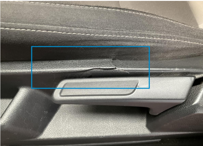
1. Seat / Front Left Interior / Broken -
