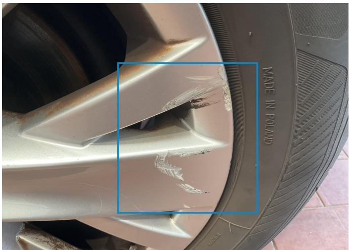
17. Rim / Back Left Out of Bodywork / Scratch -
