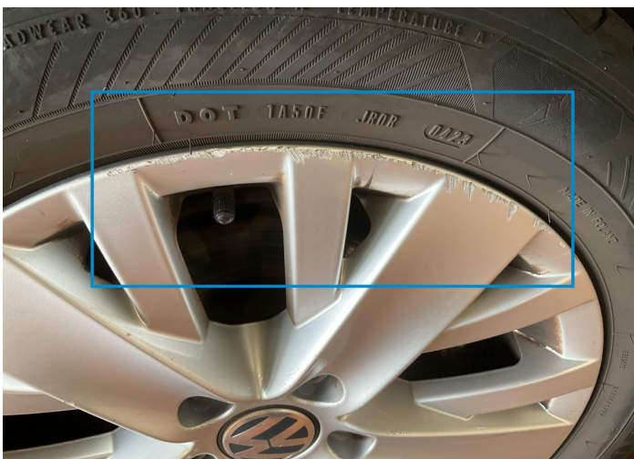
12. Rim / Back Right Out of Bodywork / Scratch -
