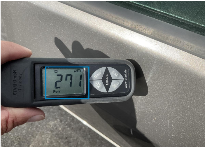
34. Door / Front Left Paint / Poor Previous Repair -
