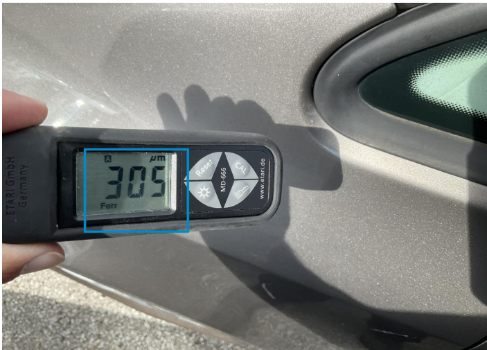
35. Fender / Front Left Paint / Poor Previous Repair -
