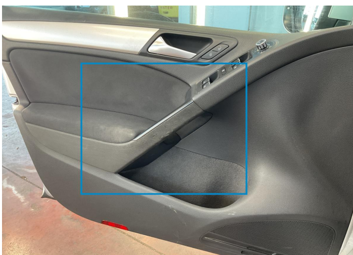
5. Panel Filling / Front Left Interior / Broken -
