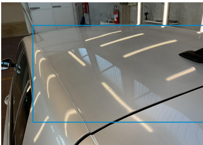
29. Roof Bodywork / Poor Previous Repair -
