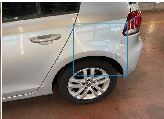
28. Fender / Back Left Bodywork / Dent -
