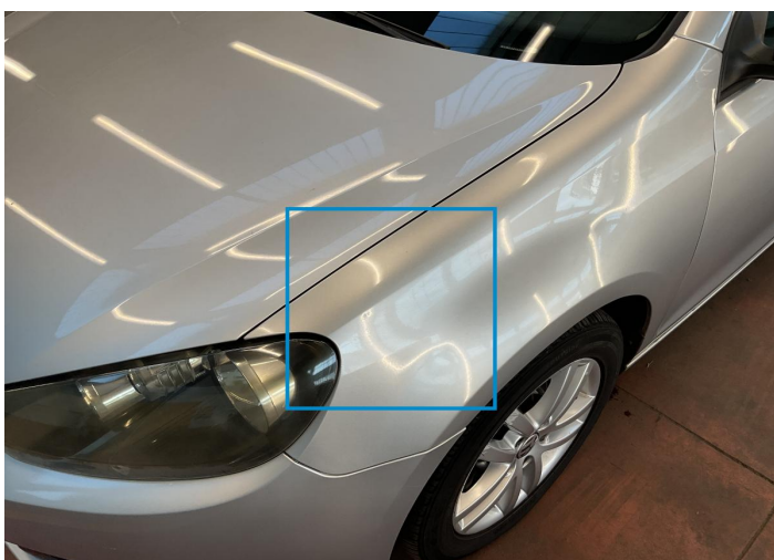
21. Fender / Front Left Bodywork / Dent -
