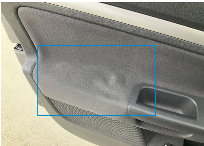
1. Panel Filling / Front Left Interior / Loose -
