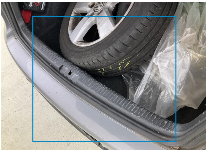
4. Ply Lining (LCV) Interior / Scratched -
