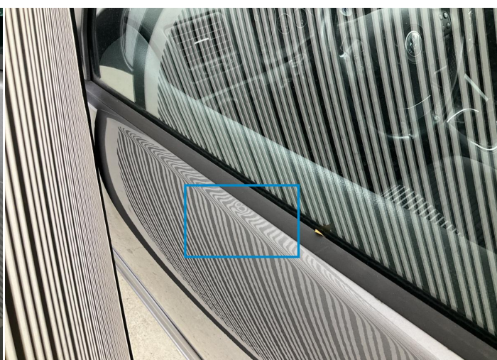
30. Door / Front Left Bodywork / Dent / Dent -
