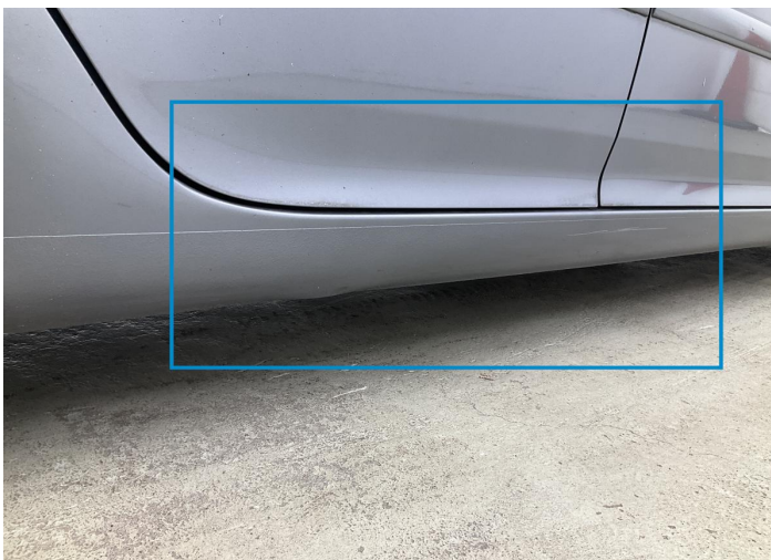
16. Rocker Panel / Center Right Bodywork / Dent / Dent -
