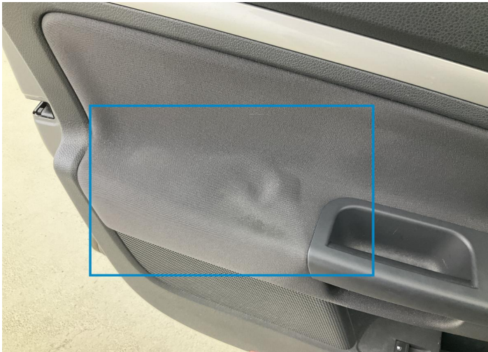
1. Panel Filling / Front Left Interior / Loose -
