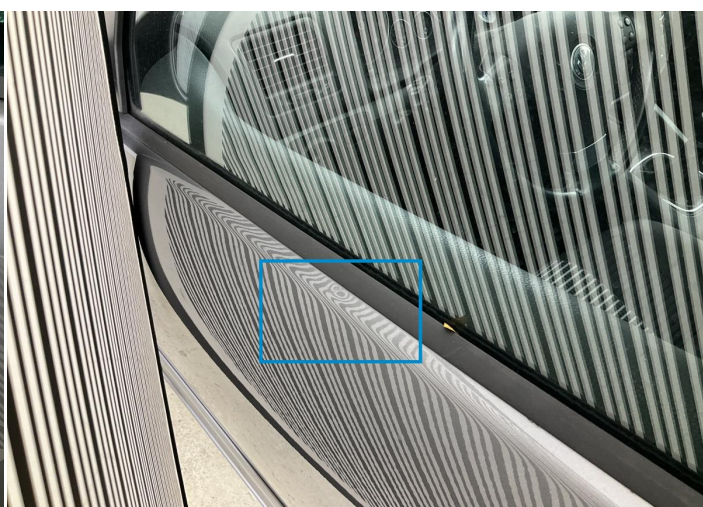
30. Door / Front Left Bodywork / Dent / Dent -
