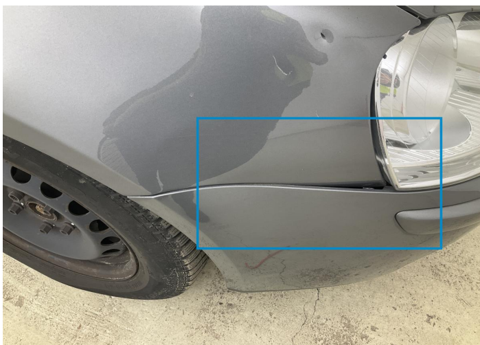
23. Fender / Front Right Bodywork / Poor Previous Repair -
