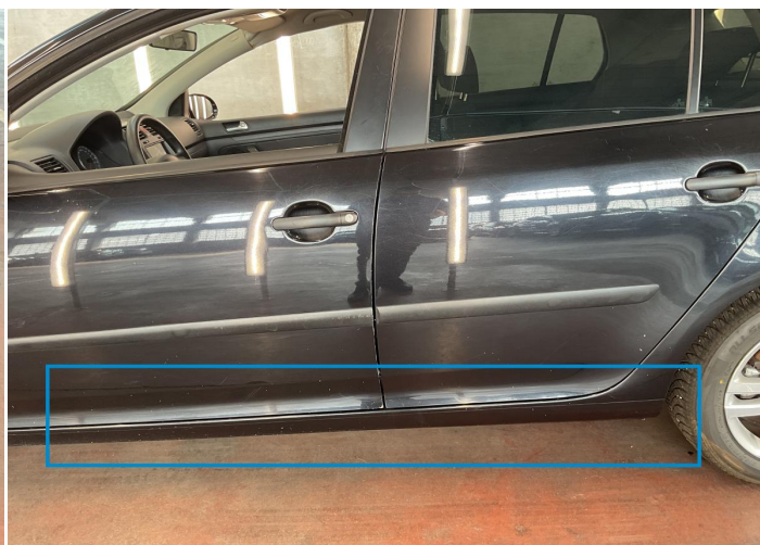
26. Rocker Panel / Center Left Paint / Chipping -
