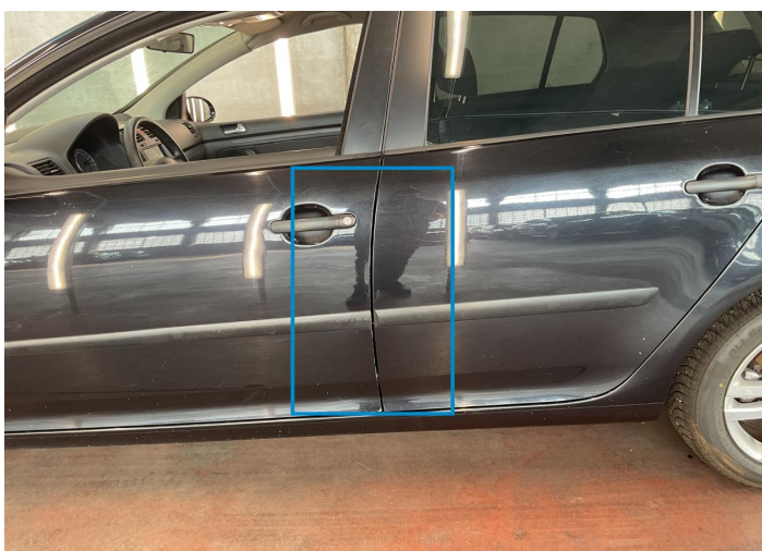
33. Door / Front Left Bodywork / Dent -
