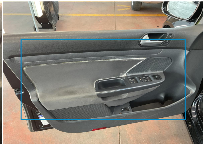
4. Panel Filling / Front Left Interior / Broken -
