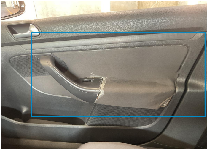
3. Panel Filling / Front Right Interior / Broken -
