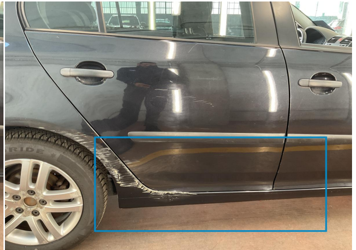
14. Rocker Panel / Center Right Bodywork / Dent -
