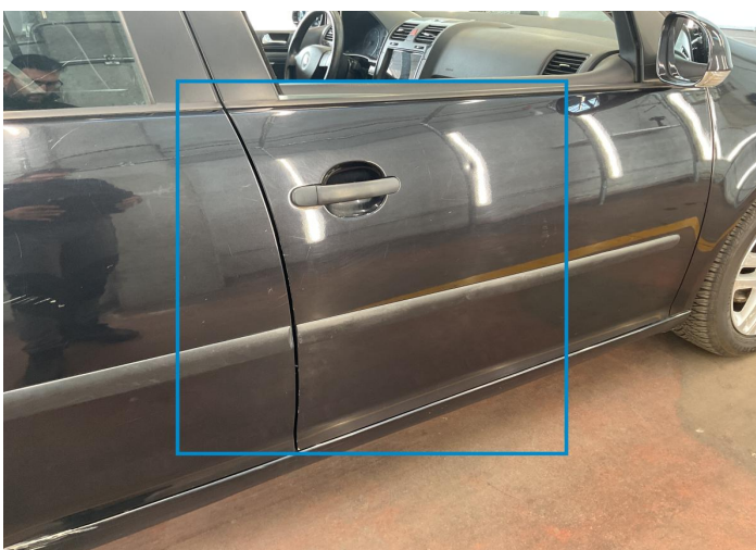
10. Door / Front Right Bodywork / Dent -
