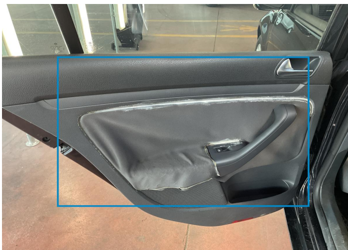
7. Panel Filling / Back Left Interior / Broken -
