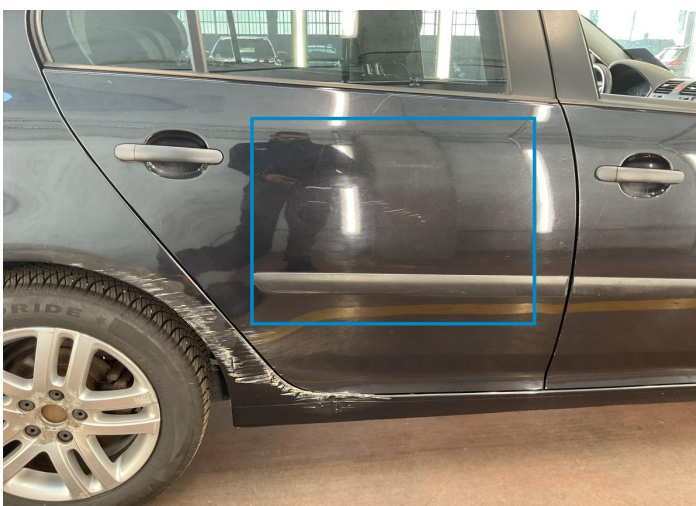
22. Door / Back Right Bodywork / Dent -
