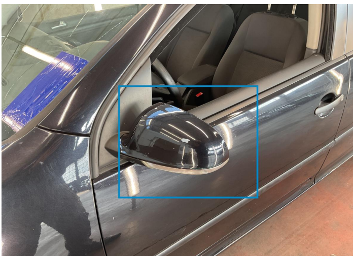
20. Mirror Shell / Front Left Bodywork / Poor Previous Repair -
