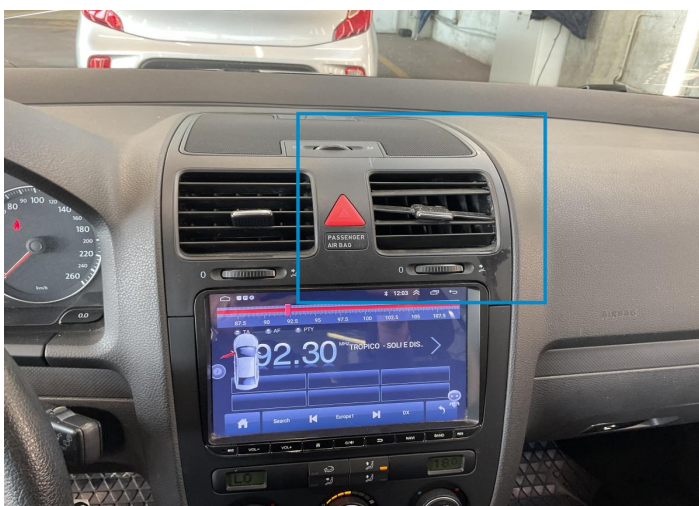
27. Aeration Grid / Front Center Interior / Broken -
