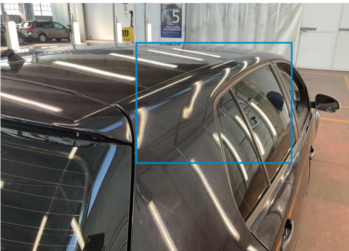
17. Pillar / Front Right Bodywork / Dent -
