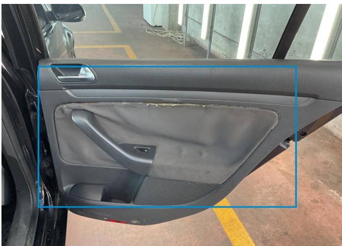
8. Panel Filling / Back Right Interior / Broken -
