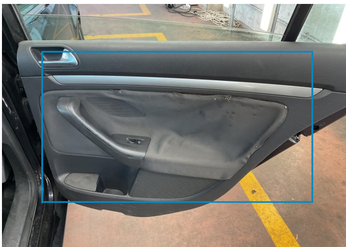
13. Panel Filling / Back Right Interior / Broken -
