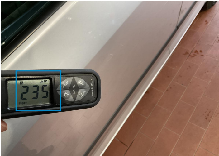
11. Door / Front Left Paint / Poor Previous Repair -
