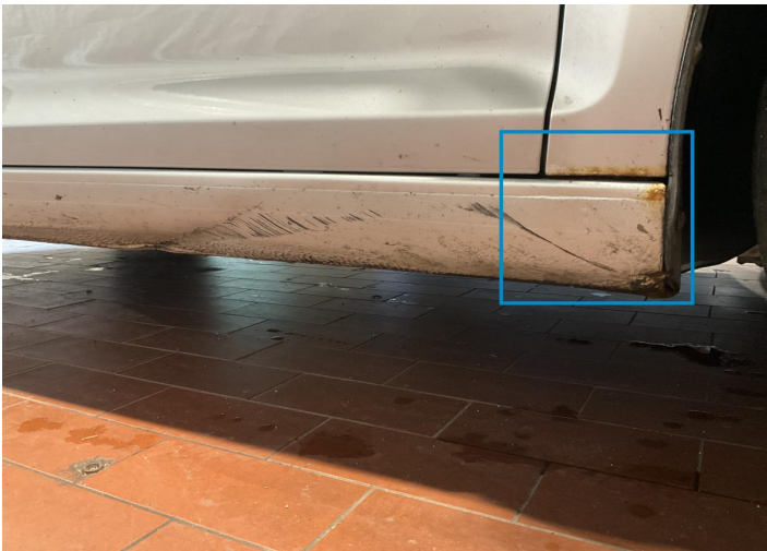
18. Rocker Panel / Center Right Paint / Chemical Damage -
