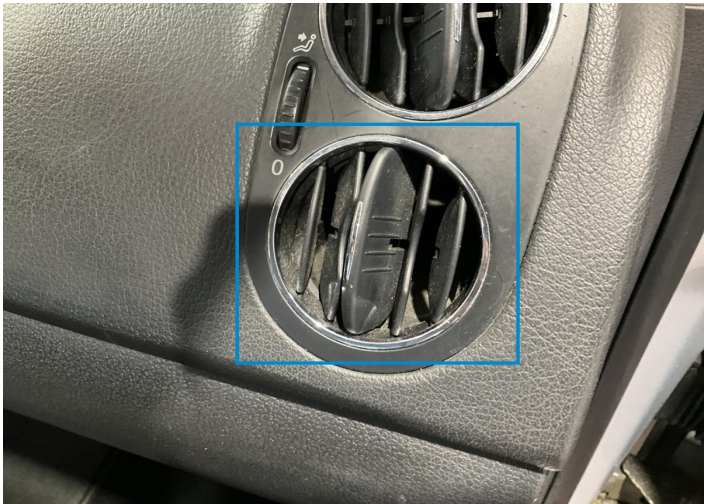
2. Aeration Grid / Front Right Interior / Broken -
