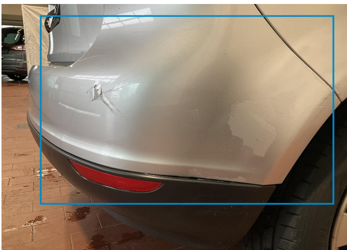
20. Bumper / Back Paint / Poor Previous Repair -
