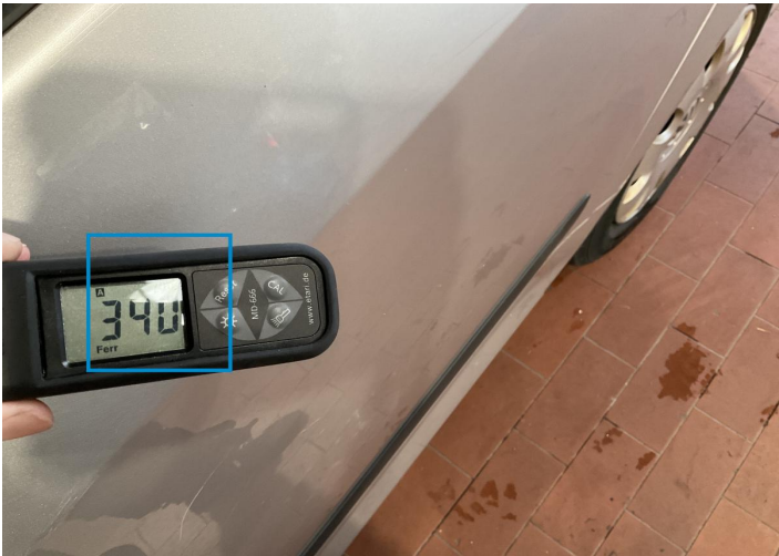
10. Door / Back Left Paint / Poor Previous Repair -
