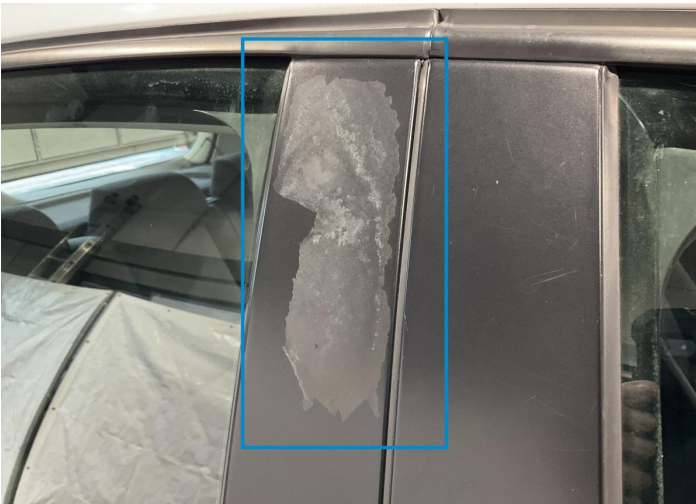
31. B Pillar / Center Right Paint / Chemical Damage -
