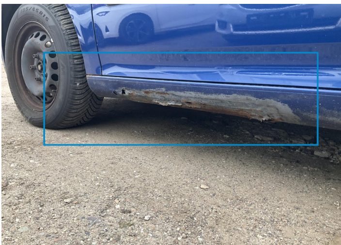
8. Rocker Panel / Center Left Paint / Corrosion -
