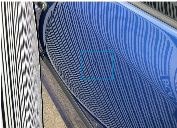
11. Fender / Back Left Bodywork / Dent / Dent -
