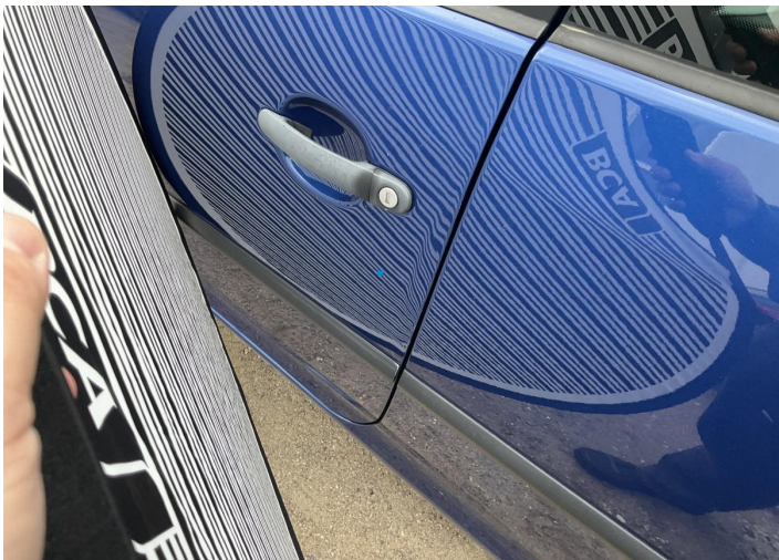
10. Door / Front Left Bodywork / Dent / Dent -
