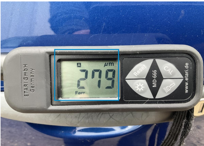
2. Door / Front Left Paint / Poor Previous Repair -
