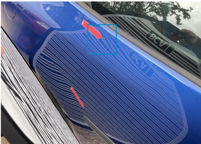
16. Fender / Back Right Bodywork / Dent / Dent -
