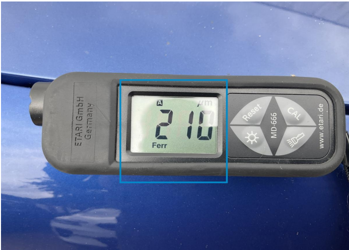
4. Fender / Front Right Paint / Poor Previous Repair -
