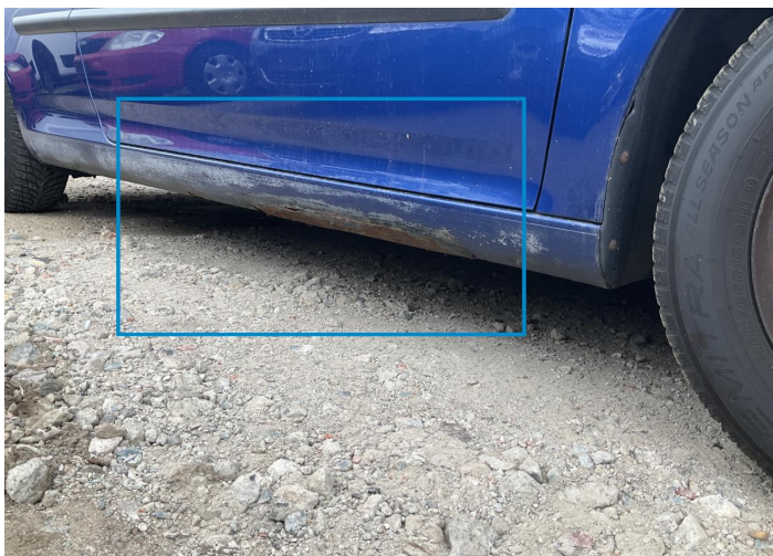
21. Rocker Panel / Center Right Paint / Corrosion -
