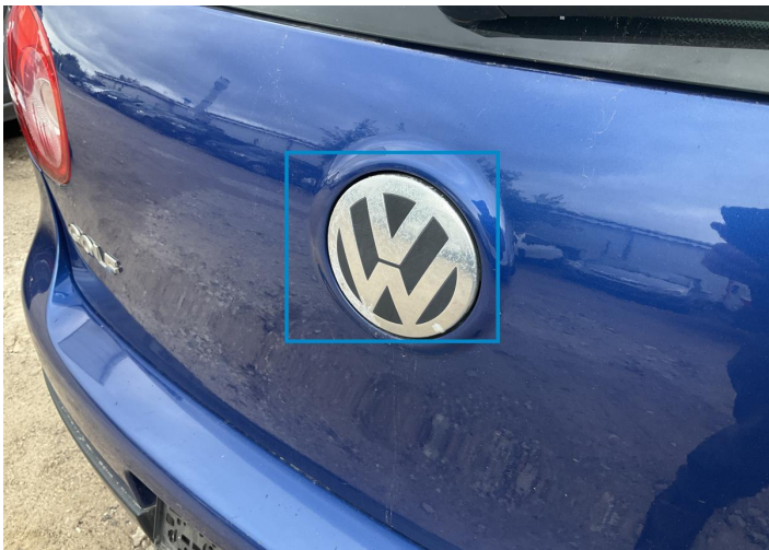
13. Monogram/Emblem / Back Center Paint / Chemical Damage -
