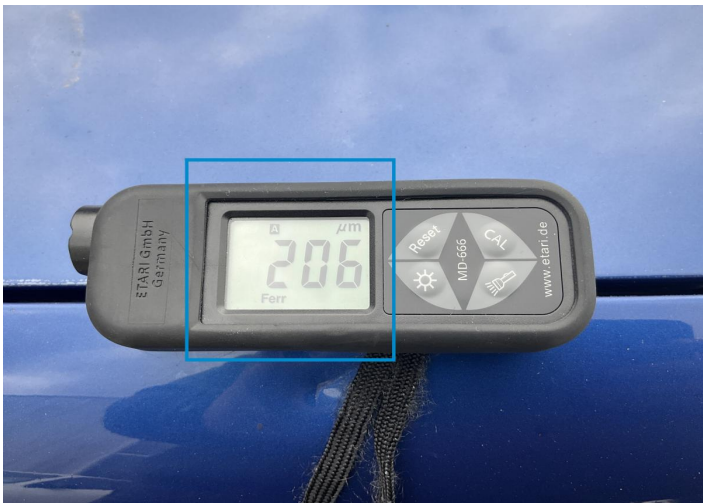
1. Fender / Front Left Paint / Poor Previous Repair -
