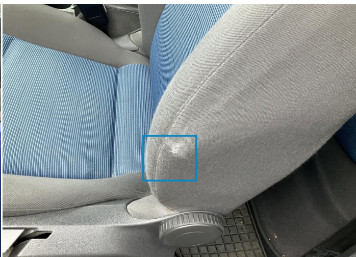
24. Seat / Front Left Interior / Ripped -
