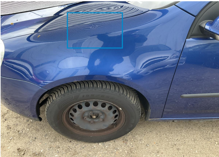
6. Fender / Front Left Bodywork / Dent / Dent -
