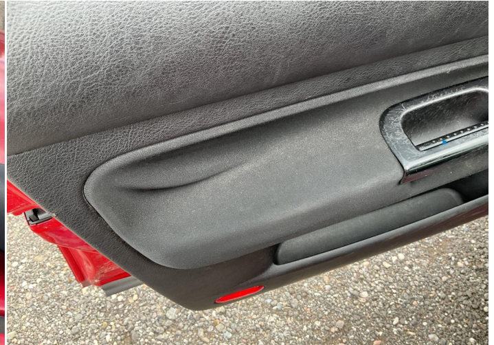
26. Panel Filling / Front Left Interior / Loose -
