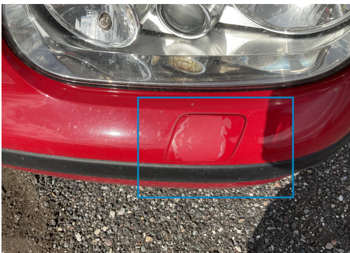
14. Shutter Cap / Front Paint / Chipping -
