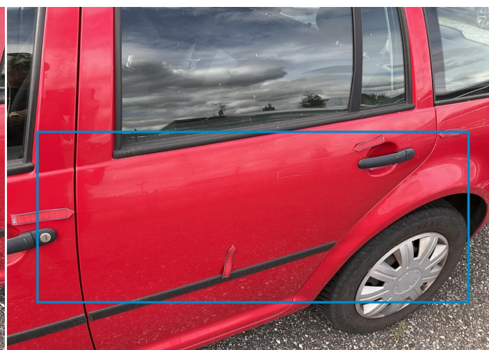
20. Door / Back Left Paint / Scratch / Scuff -
