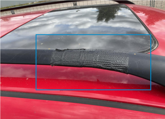
25. Bodywork / Poor Previous Repair -
