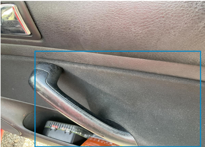
10. Panel Filling / Front Right Interior / Loose -
