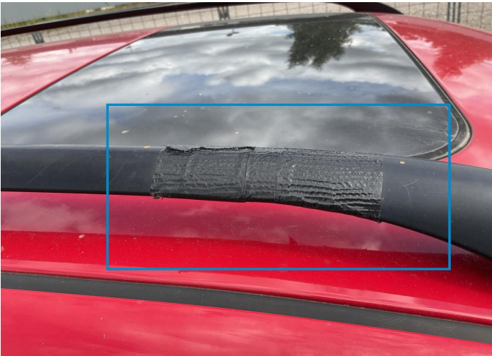
25. Bodywork / Poor Previous Repair -
