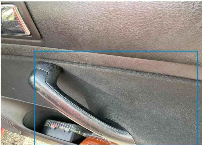
10. Panel Filling / Front Right Interior / Loose -
