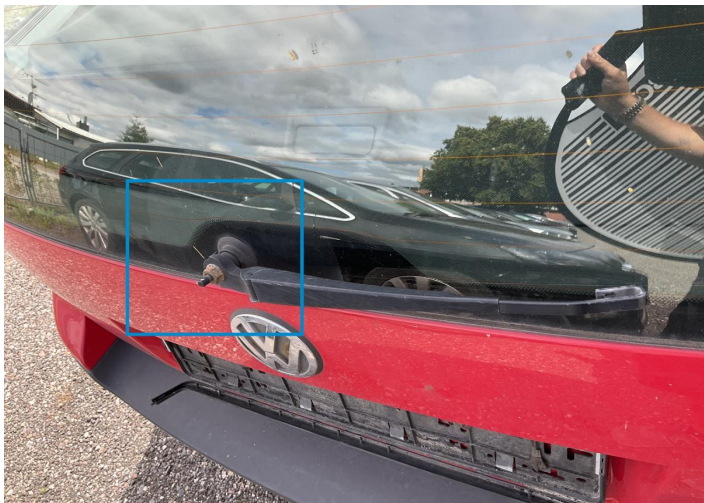
7. Wiper / Back Missing Part -
