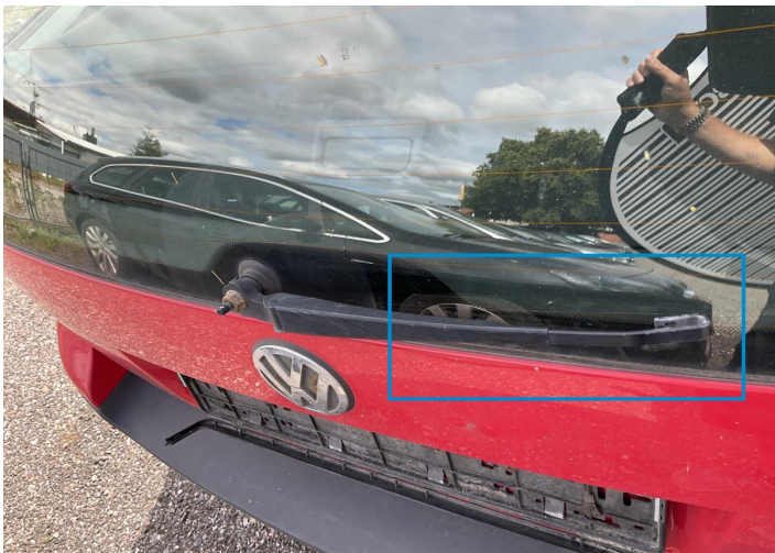
8. Wiper / Back Missing Part -
