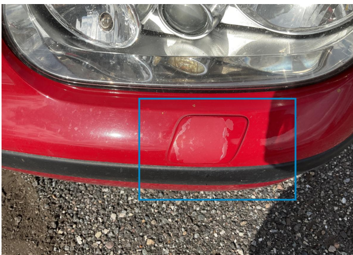
14. Shutter Cap / Front Paint / Chipping -
