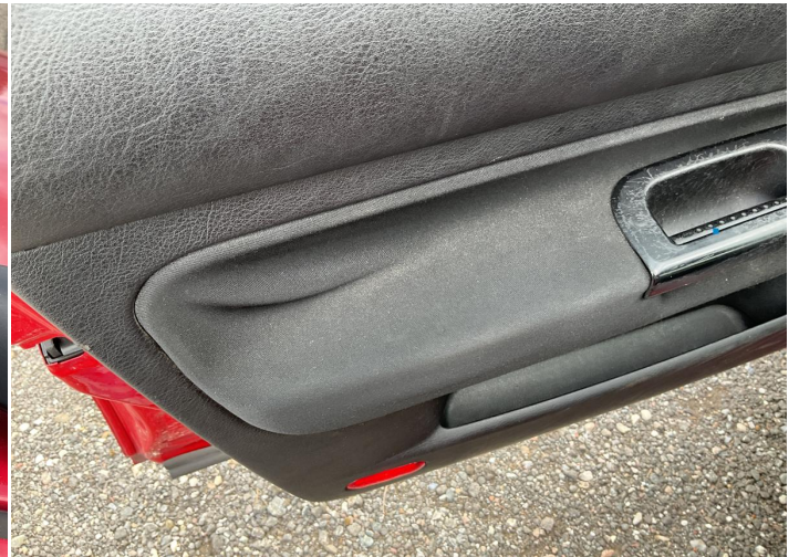
26. Panel Filling / Front Left Interior / Loose -
