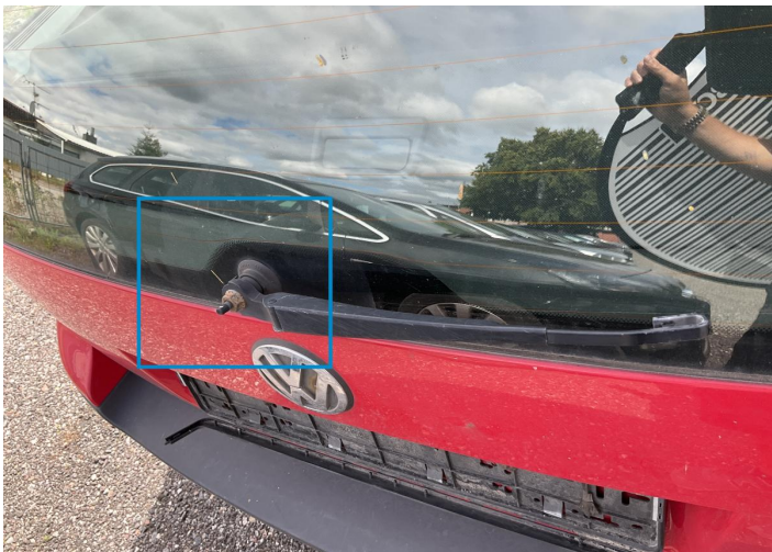
7. Wiper / Back Missing Part -
