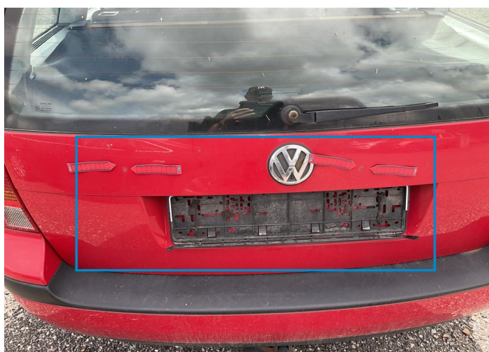
23. Tailgate Paint / Corrosion -
