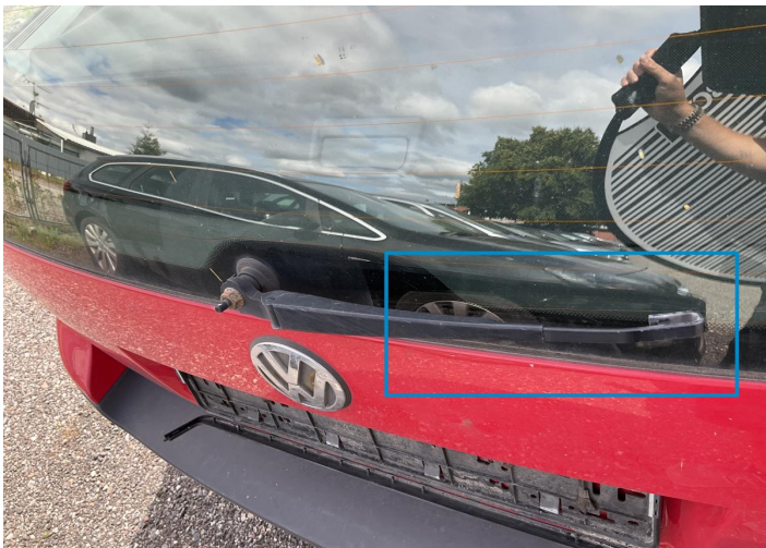
8. Wiper / Back Missing Part -
