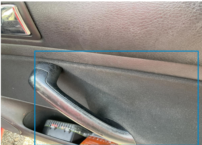
10. Panel Filling / Front Right Interior / Loose -
