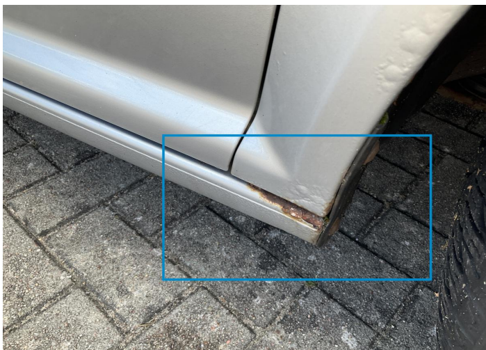
3. Rocker Panel / Center Right Paint / Chemical Damage -
