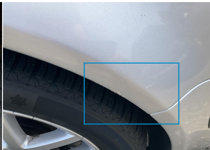
4. Fender / Front Right Paint / Chemical Damage -
