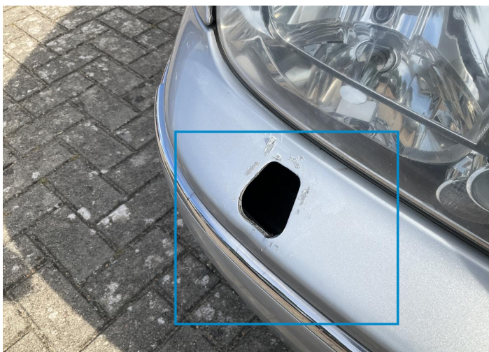
5. Headlight Nozzle / Front Right Missing Part -
