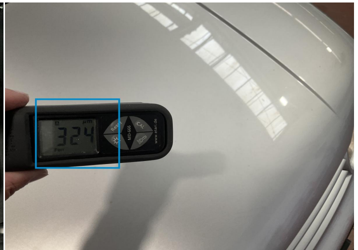
8. Hood Paint / Poor Previous Repair -
