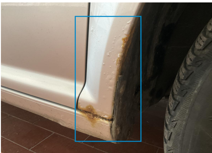
20. Fender / Front Right Paint / Chemical Damage -
