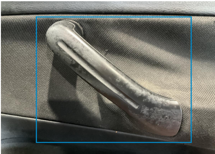
5. Panel Filling / Front Right Interior / Scratched -
