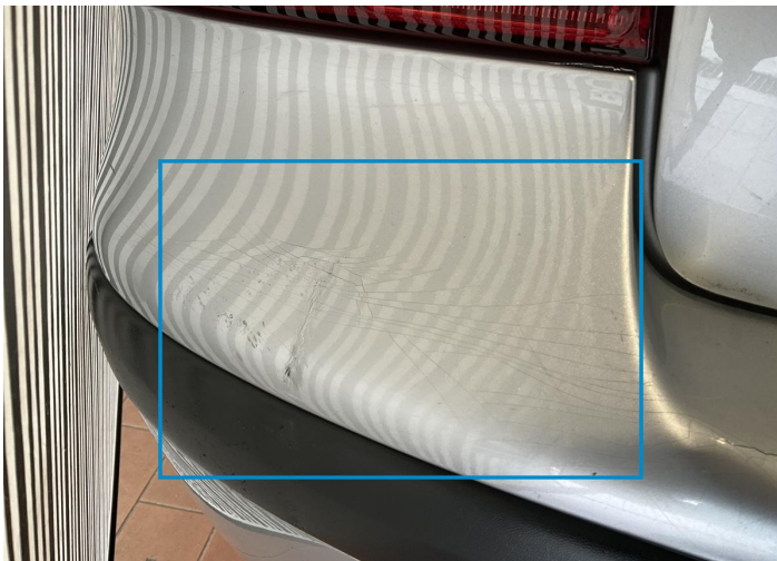
9. Bumper / Back Bodywork / Breakage / Hole -
