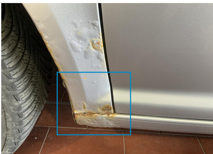
15. Rocker Panel / Center Left Paint / Chemical Damage -
