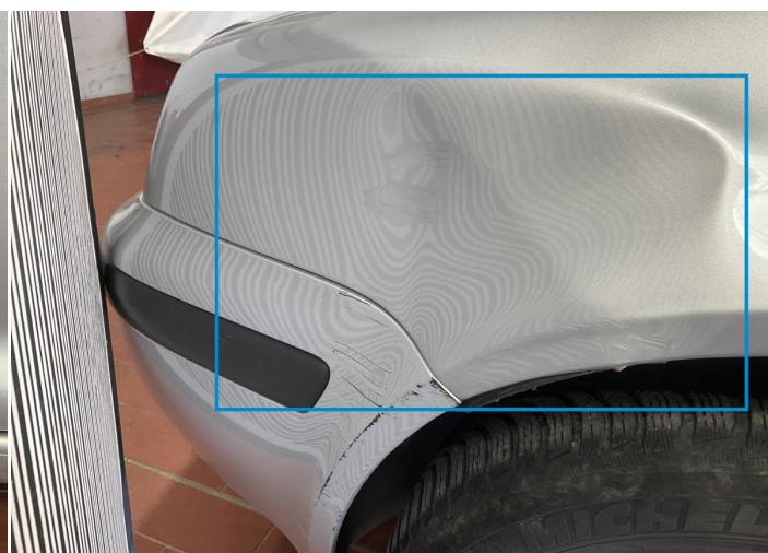
16. Fender / Front Left Bodywork / Dent / Dent -
