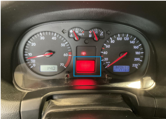
3. Digital Combined Instrument Panel Interior / Not Working -
