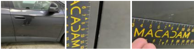
Door RR, Scratch(es), Repair and paint (complete)
