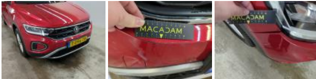
Bumper moulding F, Scratch(es), Replace and paint
