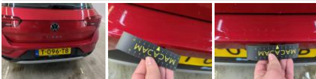
Bumper R, Scratch(es), Repair and paint (complete)
