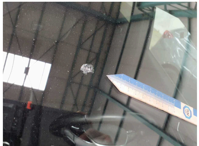
Damage 4: Vehicle glazing: Windscreen - Stone chips - Replace
