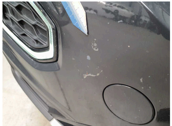
Damage 2: Front bumper: Front bumper - Paint defect - Paint
