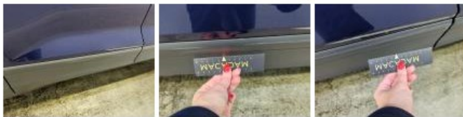
Door FR, Scratch(es), Repair and paint (complete)
