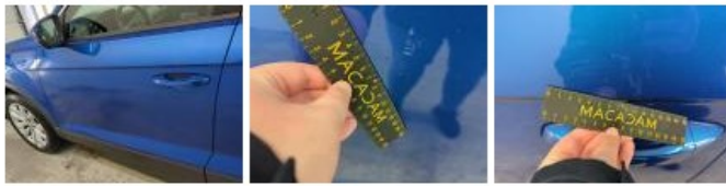
Door RL, Scratch(es), Repair and paint (complete)
