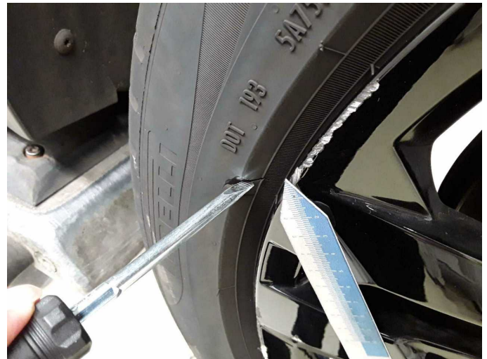
Damage 10: Wheel / tyres: Tyre - front right side (nicht fahrbereit) - Broken / torn - Replace
