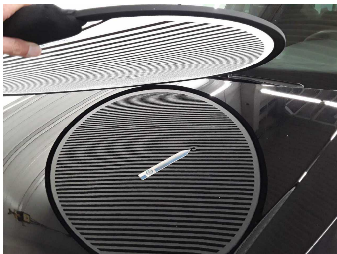
Damage 5: Bonnet: Bonnet (2x) - dent(s) - Smooth repair work
