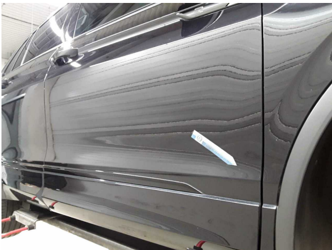
Damage 9: Door - front right side: Door - Scratch(es) - Smart repair
