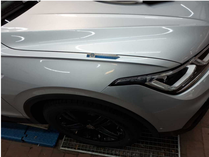
Damage 1: Mudguard - right side: Mudguard - right side - Stone chips - Smart repair
