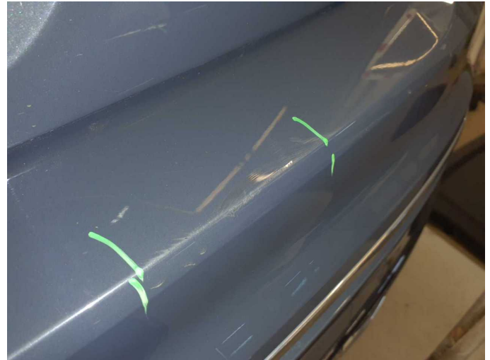
Damage 1: Rear bumper: Rear bumper - Scratch(es) - Paint
