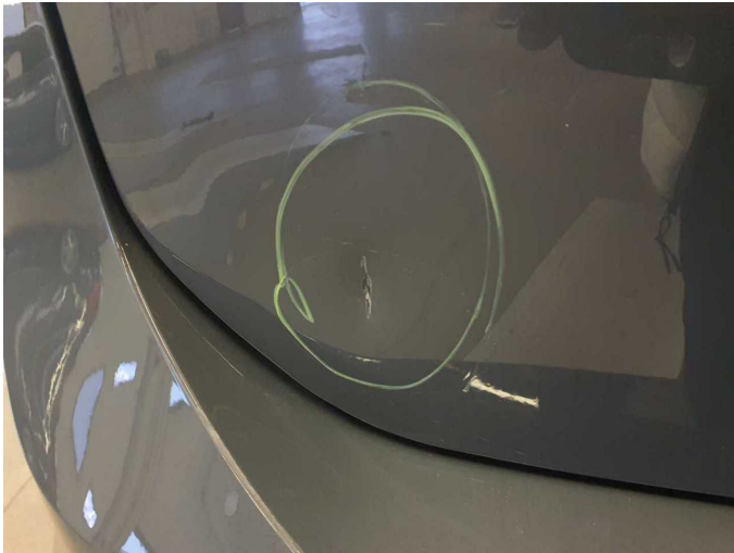
Damage 4: Boot lid / rear door: Boot lid - Deformed - Repair and paint
