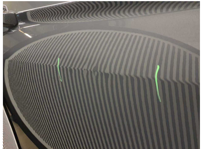
Damage 3: Door - front right side: Door - Unprofessionally repaired - Repair and paint
