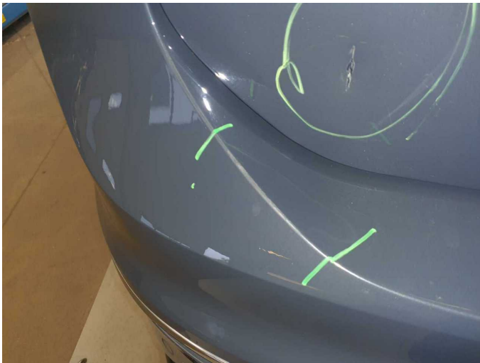
Damage 1: Rear bumper: Rear bumper - Scratch(es) - Paint
