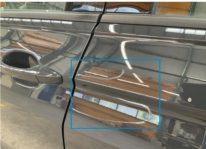
5. Door / Back Left Paint / Scratch / Scuff -
