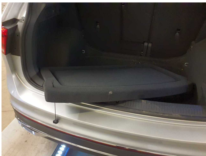
Damage 12: Interior: Rear shelf - Broken / torn - Replace
