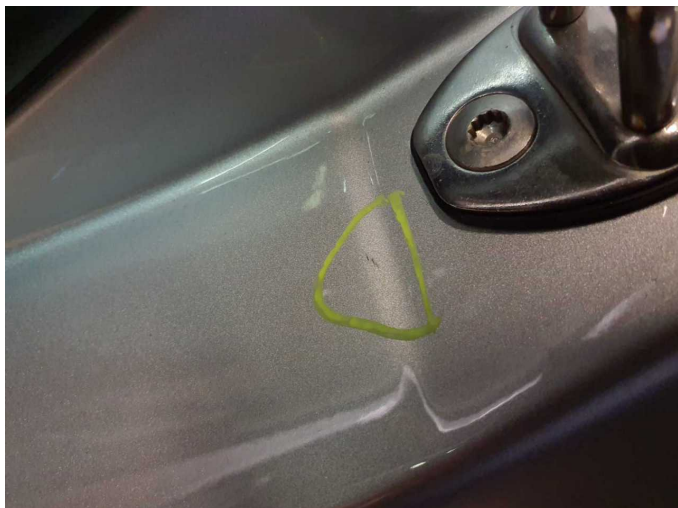
Damage 11: Side panel - rear left side: Sill - Scratched - Smart repair
