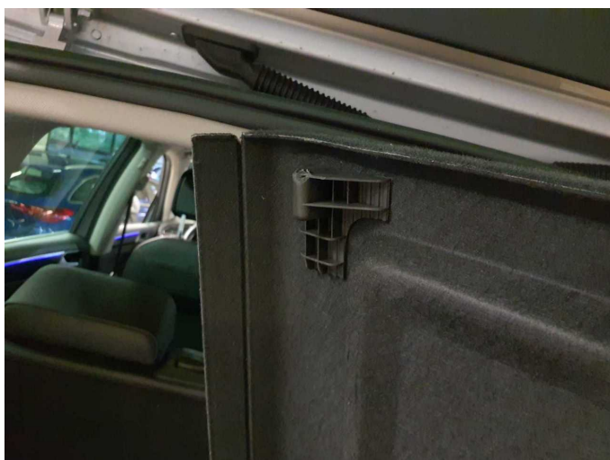
Damage 12: Interior: Rear shelf - Broken / torn - Replace
