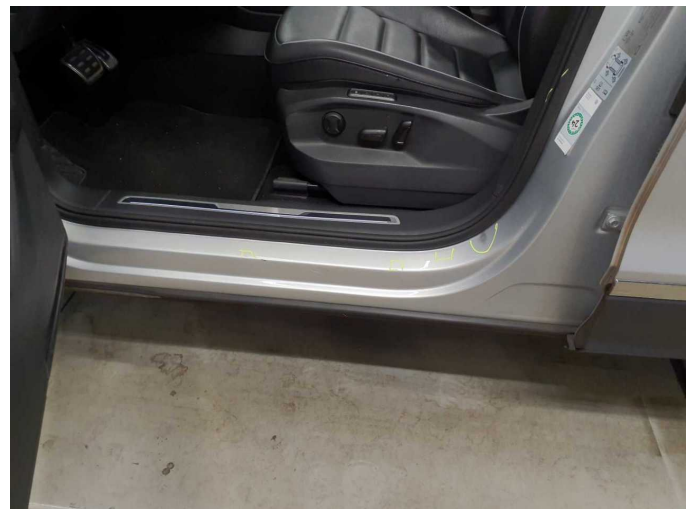
Damage 10: Sill - left side: Sill (Lackfehler / Lackpickel / Kratzer) - Scratched - Smart repair
