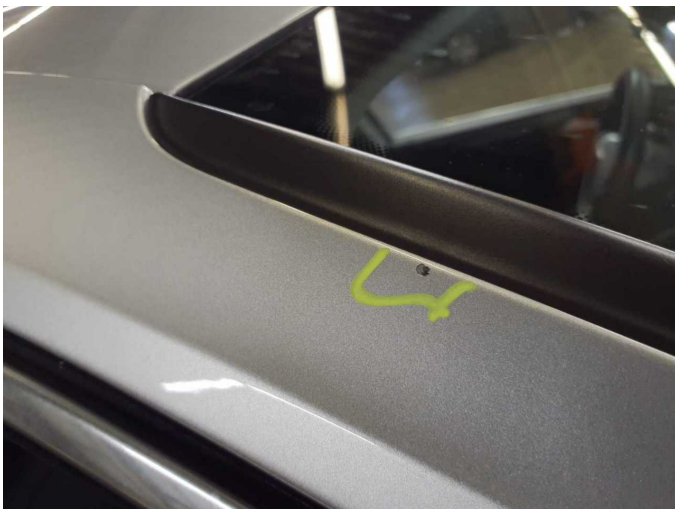
Damage 9: Roof: Roof rail - right side - Stone chips - Smart repair
