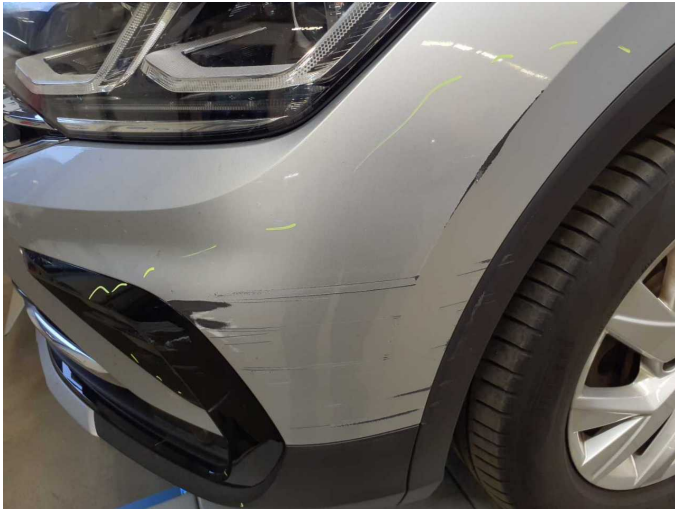
Damage 13: Front bumper: Front bumper - Scratched - Paint
