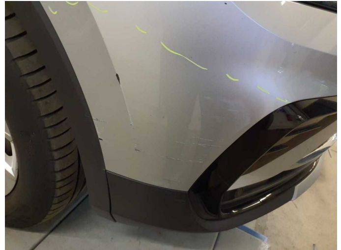
Damage 13: Front bumper: Front bumper - Scratched - Paint
