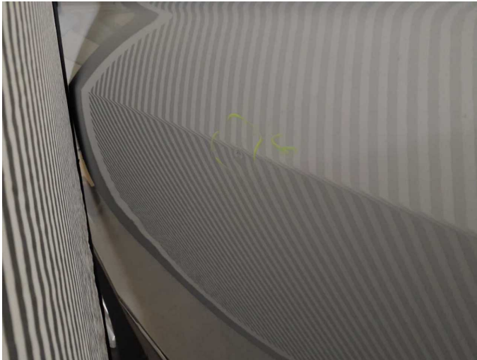
Damage 7: Door - rear right side: Door - dent(s) - Smooth repair work
