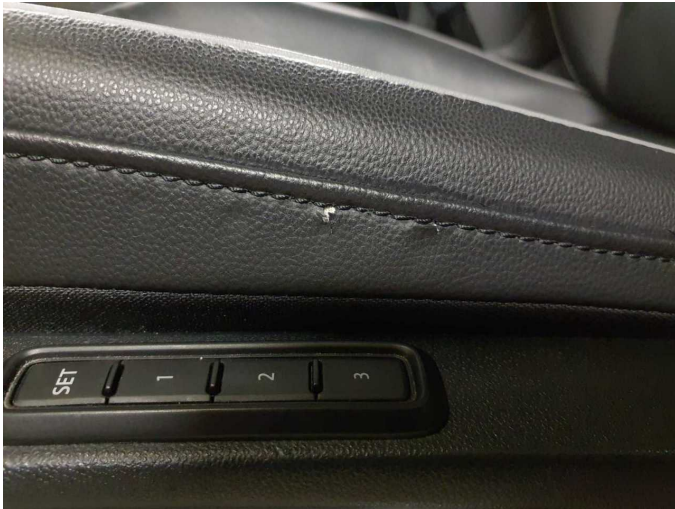
Damage 8: Seat - front: Seat cover - left side - Scratched - Smart repair
