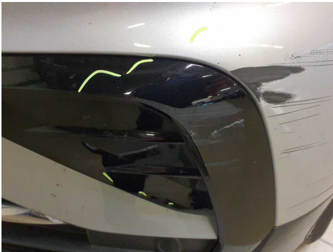
Damage 13: Front bumper: Front bumper - Scratched - Paint
