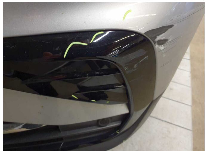
Damage 14: Front bumper: Cover bumper - front (Materialabtrag) - Scratched - Replace
