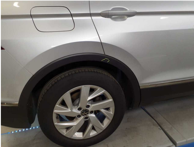
Damage 5: Side panel - rear right side: Wheel well extension - Scratch(es) - Loss in value
