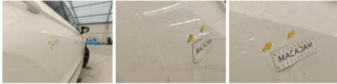
Door FR, Dent(s), Repair and paint (complete)
