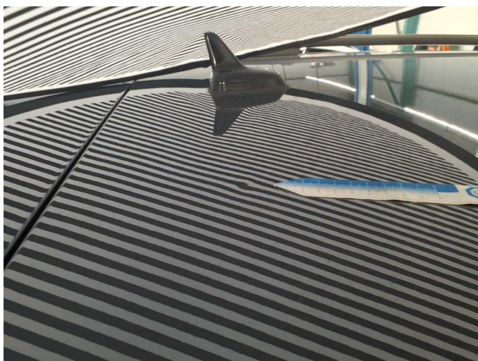
Damage 3: Roof: Roof - dent(s) - Smooth repair work
