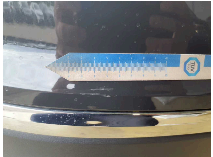
Damage 12: Rear bumper: Rear bumper - Scratch(es) - Paint
