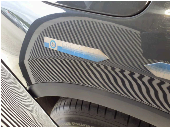
Damage 14: Side panel - rear right side: Side panel (Wellig) - Unprofessionally repaired - Repair and paint
