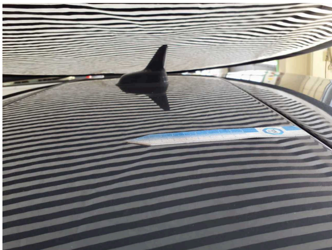
Damage 4: Roof: Roof - dent(s) - Smooth repair work
