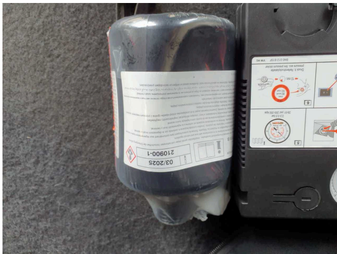
Damage 1: Equipment: Tirefit filler - Expired - Replace
