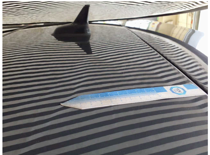
Damage 4: Roof: Roof - dent(s) - Smooth repair work
