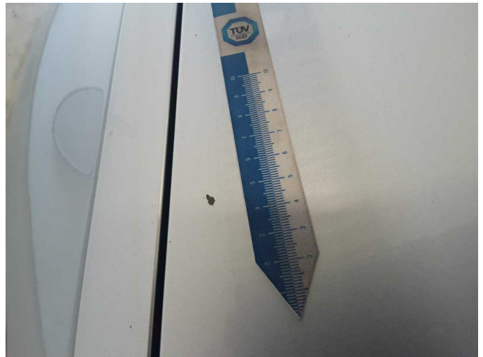
Damage 2: Bonnet: Bonnet - Stone chips - Paint
