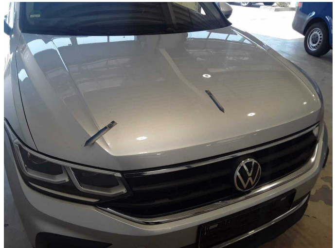
Damage 2: Bonnet: Bonnet - Stone chips - Paint
