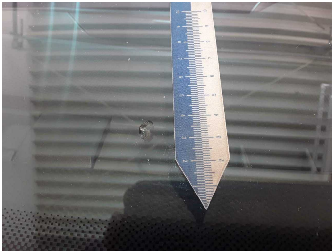
Damage 3: Vehicle glazing: Windscreen - Damaged - Replace
