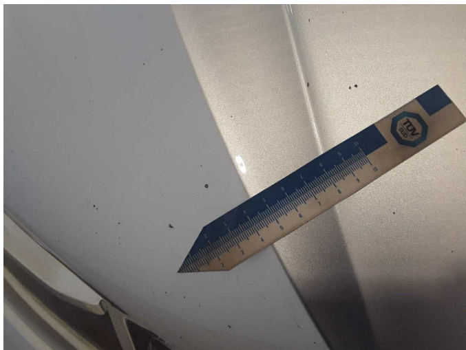
Damage 2: Bonnet: Bonnet - Stone chips - Paint
