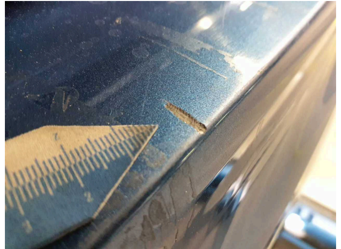
Damage 22: Rear bumper: Rear bumper - Scratched - Repair and paint
