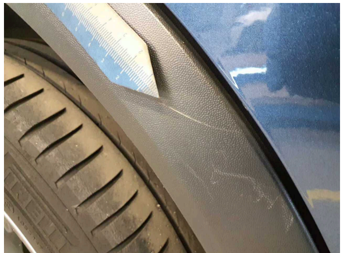
Damage 14: Side panel - rear right side: Wheel well extension - Scratched - Replace
