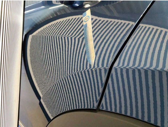
Damage 7: Door - rear left side: Door (Steinschlag) - Scratched - Smart repair
