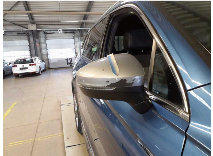
Damage 4: Wing mirror - right side: Cap - Scratched - Paint
