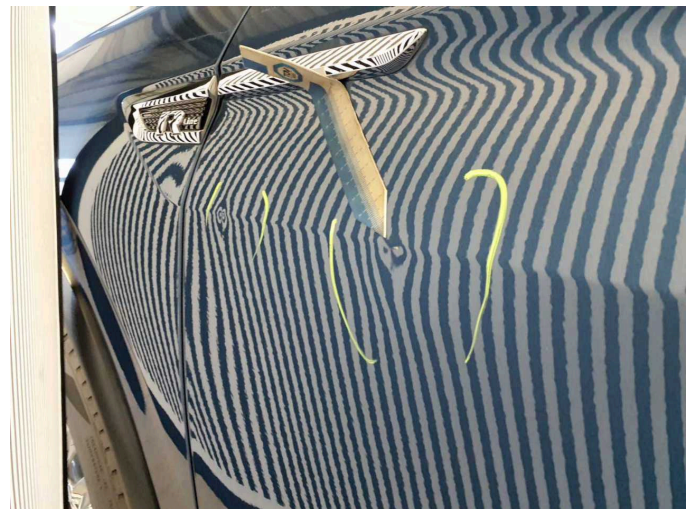
Damage 23: Door - front left side: Door - Dent / paintcoat damage - Repair and paint
