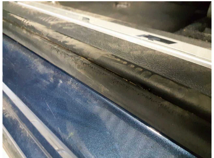
Damage 13: Door - front left side: Door seal - Scratched - Replace
