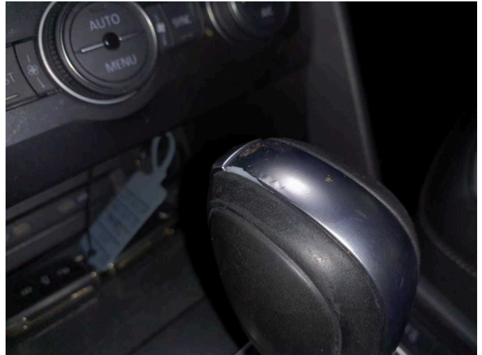
Damage 15: Gearbox: Gear knob - Scratched - Replace
