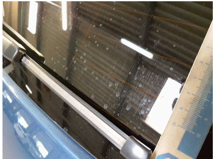
Damage 16: Vehicle glazing: Rear window - Scratched - Loss in value
