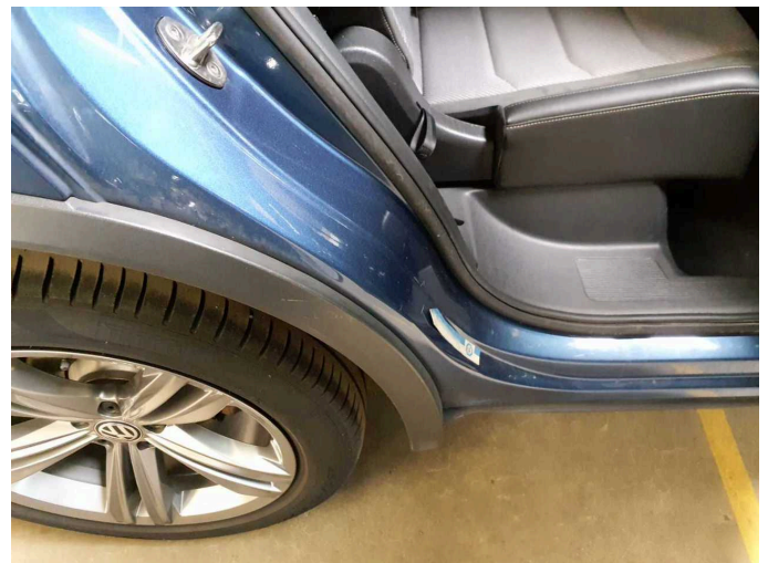
Wear and tear 17: Side panel - rear right side: Sill - Scratch(es) - Cover / polish
