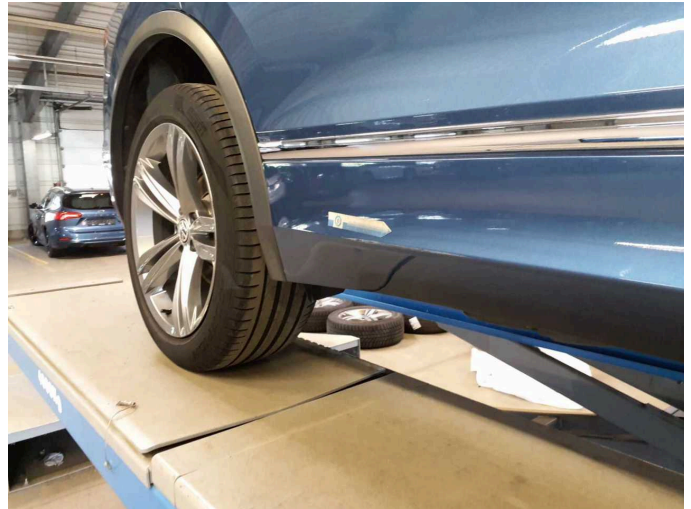
Damage 10: Door - rear right side: Brightware - lower - Scratched - Paint
