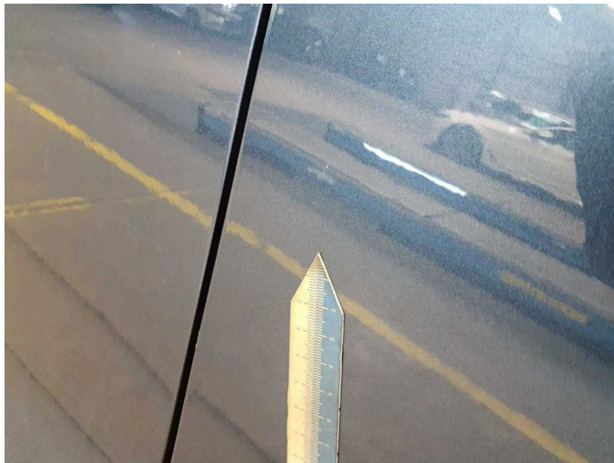
Wear and tear 7: Door - front right side: Door - Paint defect - No deduction
