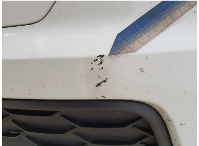
Damage 5: Front bumper: Front bumper - Scratch(es) - Paint
