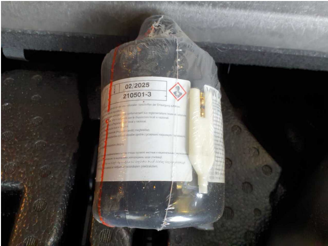
Damage 1: Equipment: Tirefit filler - Expired - Replace
