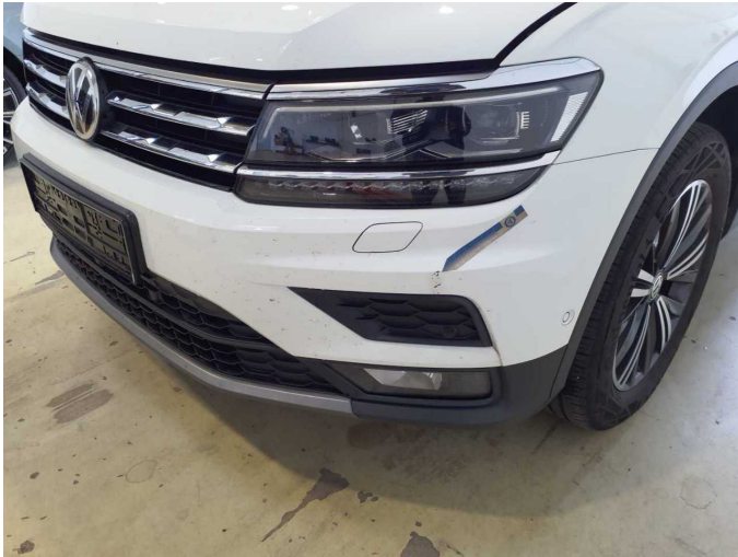
Damage 5: Front bumper: Front bumper - Scratch(es) - Paint
