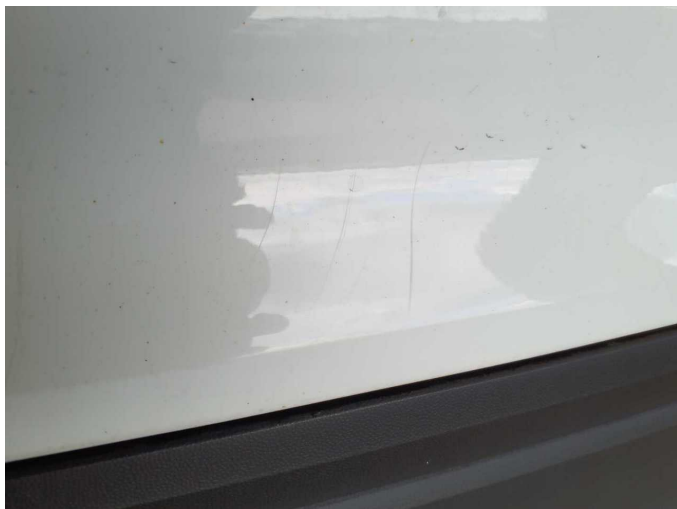
Damage 4: Rear bumper: Rear bumper - Scratch(es) - Paint
