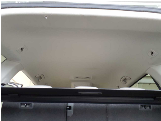
Damage 7: Trim / covers: Roof lining - Damaged - Replace
