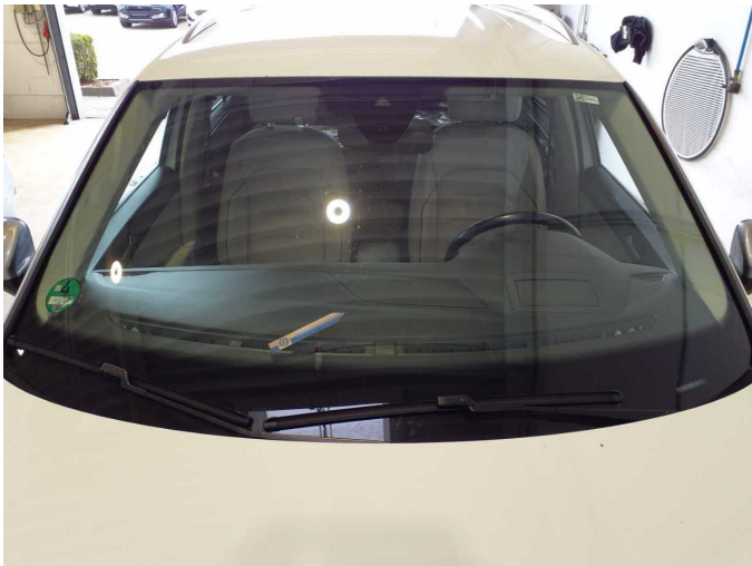
Damage 6: Vehicle glazing: Windscreen with lane departure assistant - Damaged - Replace
