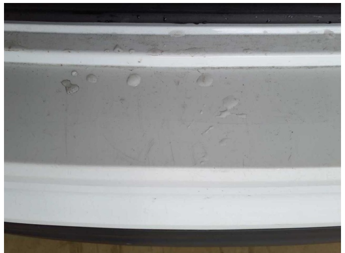
Damage 4: Rear bumper: Rear bumper - Scratch(es) - Paint
