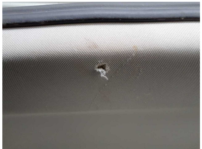
Damage 7: Trim / covers: Roof lining - Damaged - Replace
