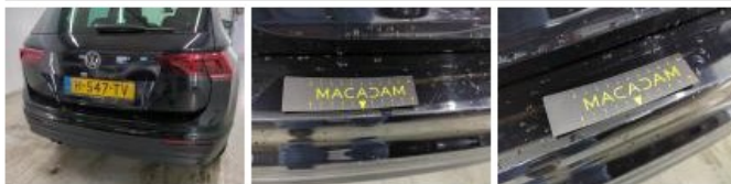
Tailgate / Boot, Scratch(es), Repair and paint (complete)
