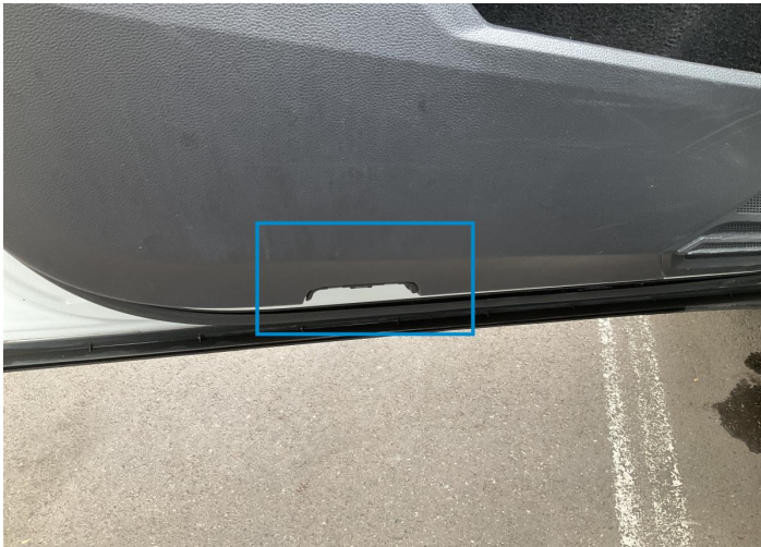
9. Panel Filling / Front Left Interior / Missing -
