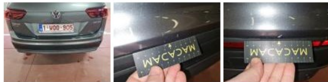
Bumper moulding R, Dent(s) and scratch(es), Replace
