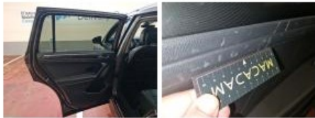
Door panel RR, Scratch(es), Smart repair
