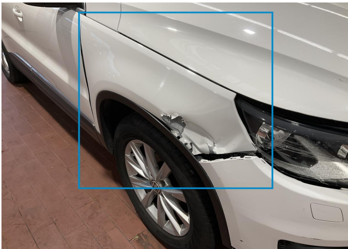
1. Fender / Front Right Bodywork / Dent / Dent -
