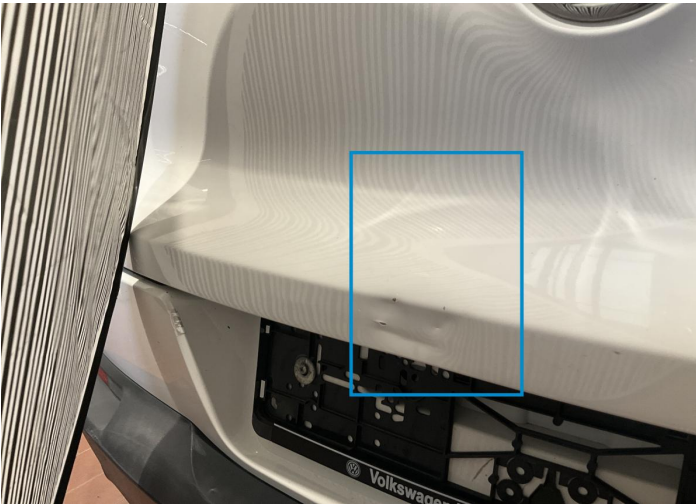
9. Rear Trunk Bodywork / Dent / Dent -
