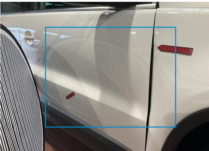
11. Door / Front Right Bodywork / Dent / Dent -
