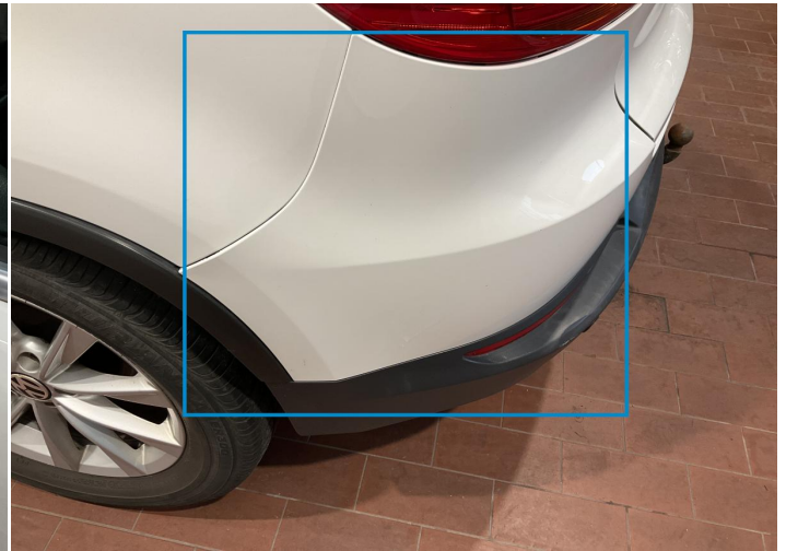
8. Bumper / Back Bodywork / Breakage / Crack -
