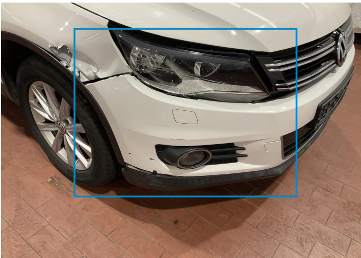
2. Bumper / Front Bodywork / Breakage / Crack -
