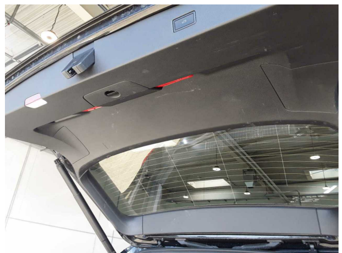
Damage 2: Boot lid / rear door: Trim - standard - lower - Scratched - Replace
