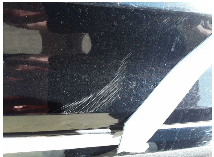
Damage 4: Rear bumper: Rear bumper - Scratched - Paint
