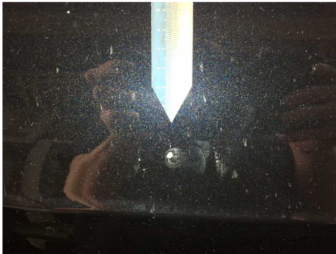
Damage 9: Bonnet: Bonnet - Stone chips - Repair and paint
