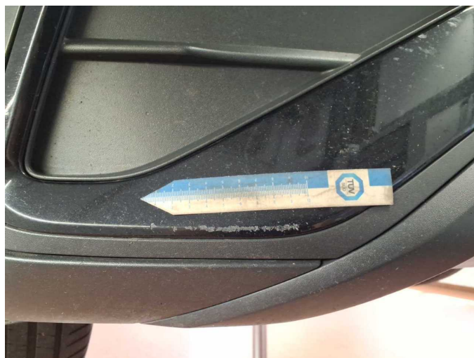
Damage 8: Front bumper: Front bumper - Scratched - Paint
