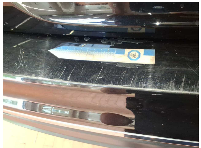
Damage 7: Rear bumper: Rear bumper - Scratched - Paint
