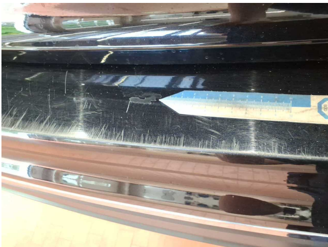
Damage 7: Rear bumper: Rear bumper - Scratched - Paint
