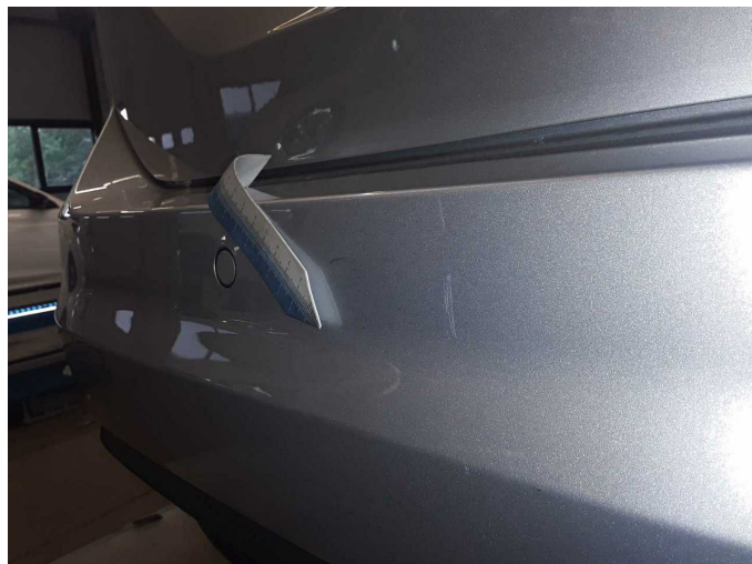
Damage 3: Rear bumper: Rear bumper - Scratch(es) - Paint
