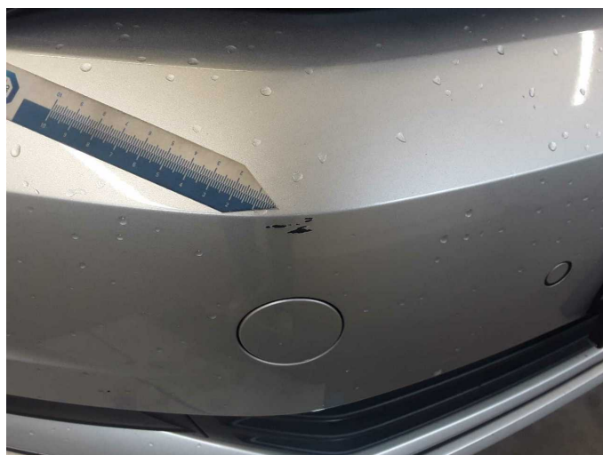
Damage 4: Front bumper: Front bumper - Scratch(es) - Paint
