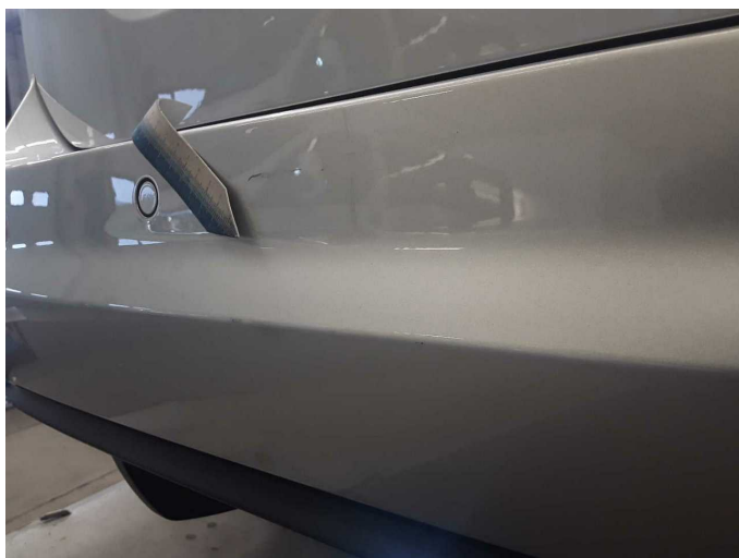
Damage 3: Rear bumper: Rear bumper - Scratch(es) - Paint
