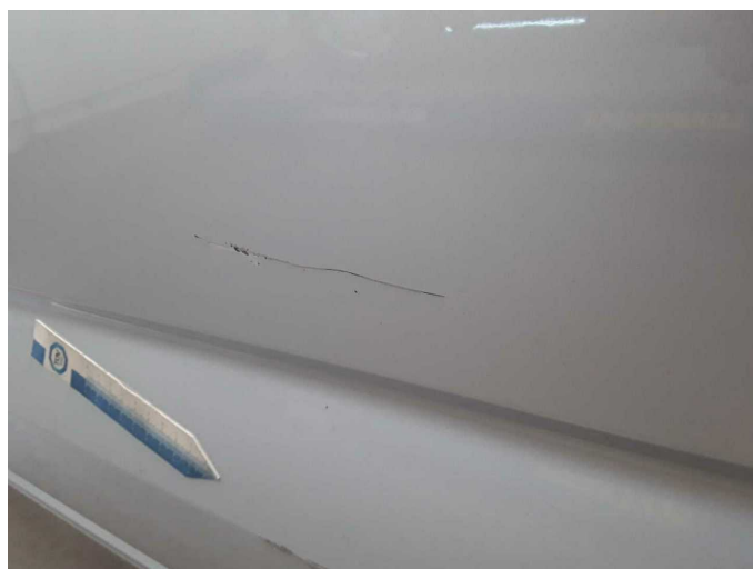
Damage 2: Door - front left side: Door - Scratched - Paint
