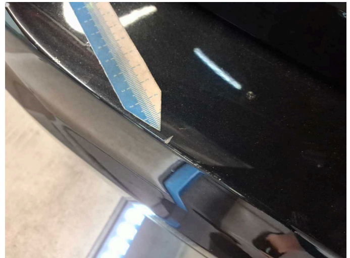
Damage 4: Rear bumper: Rear bumper - Scratch(es) - Paint
