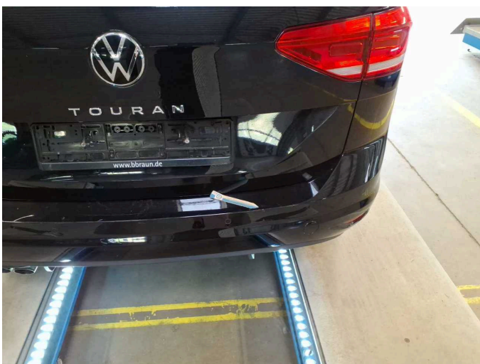
Damage 4: Rear bumper: Rear bumper - Scratch(es) - Paint
