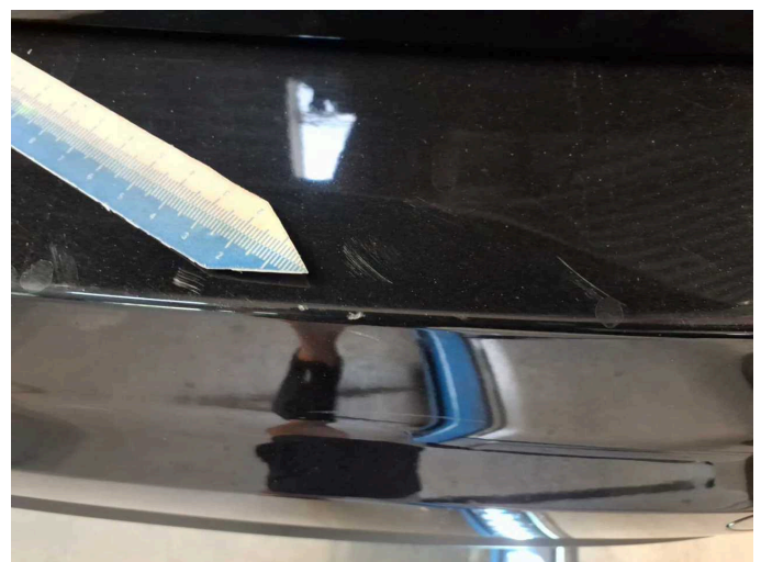
Damage 4: Rear bumper: Rear bumper - Scratch(es) - Paint
