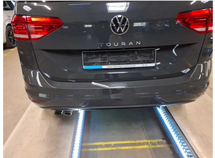
Damage 8: Rear bumper: Rear bumper - Scratch(es) - Paint
