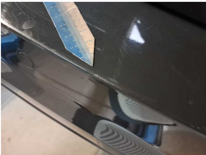
Damage 8: Rear bumper: Rear bumper - Scratch(es) - Paint
