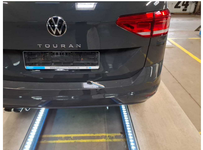
Damage 8: Rear bumper: Rear bumper - Scratch(es) - Paint
