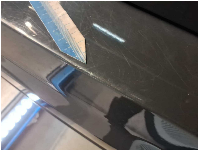
Damage 8: Rear bumper: Rear bumper - Scratch(es) - Paint
