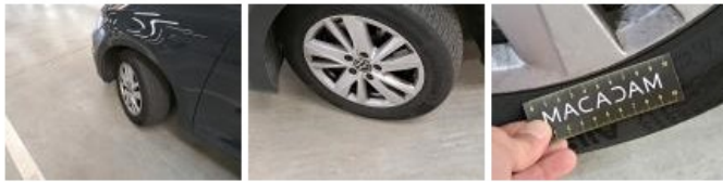
Tyre FR, Out of tolerance, Replace
