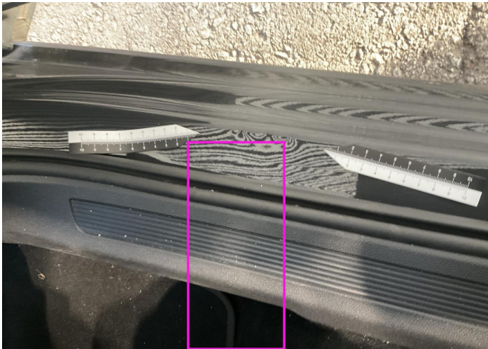
4. Rocker Panel / Center Right Bodywork / Dent / Dent -
