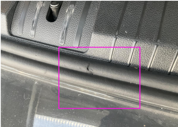
3. Bodywork / Breakage / Crack -
