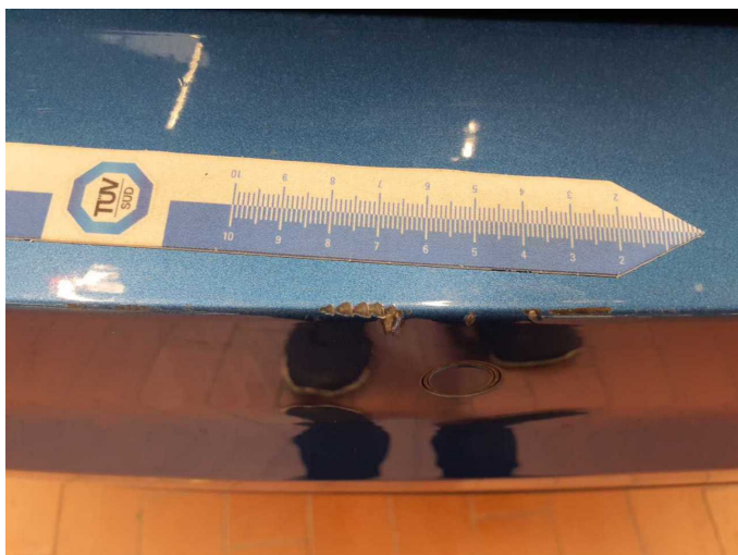
Damage 9: Rear bumper: Rear bumper - Scratch(es) - Paint
