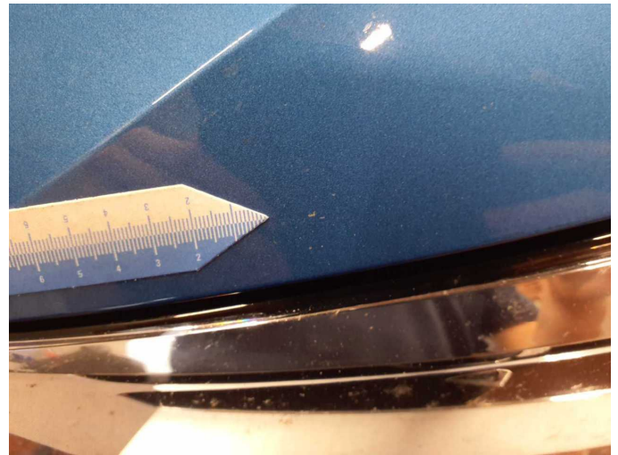
Damage 8: Bonnet: Bonnet - Stone chips - Paint
