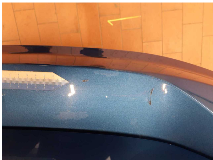
Damage 9: Rear bumper: Rear bumper - Scratch(es) - Paint
