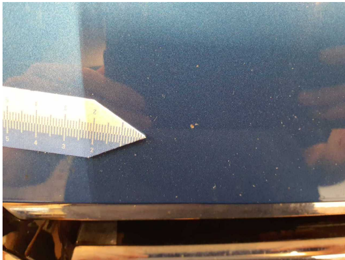
Damage 8: Bonnet: Bonnet - Stone chips - Paint
