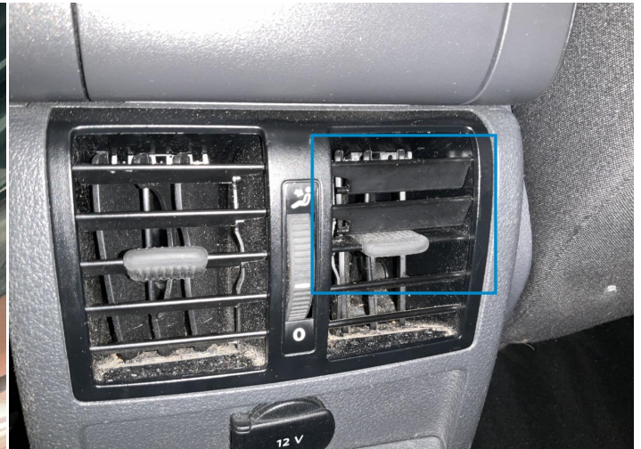
4. Aeration Grid / Back Center Interior / Broken -
