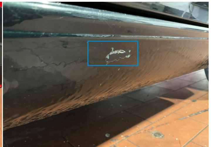
6. Rocker Panel / Center Right Paint / Stone Chip -
